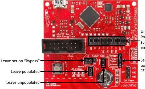
Unpopulate all if using external power. Populate GND, V+, RST, and TST if supplying power through the eZ-FET and debugging or using EnergyTrace
