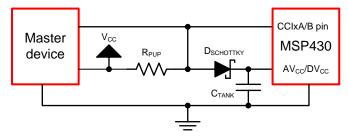
Figure 1. TIDM-1WIREFREEPROM System Block Diagram
