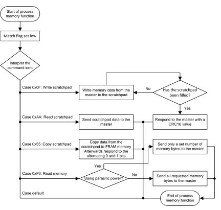
Figure 7. Memory Command Function Block Diagram
