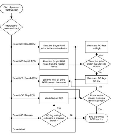
Figure 6. ROM Command Function Block Diagram
