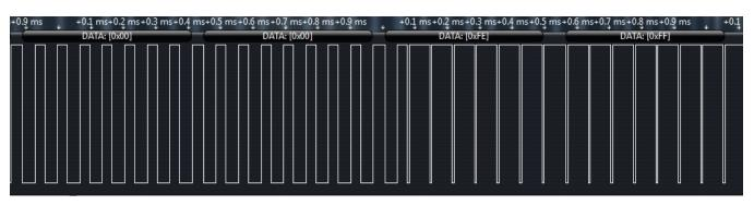
Figure 13. Parasitic Power Operation  $C_{Tank}$  Drain Example
