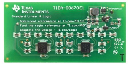
Figure 6. Top View of AA Battery Tester
