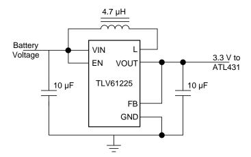
Figure 4. TLV61225 Application Schematic
