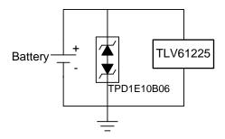
Figure 5. TPD1E10B06 Application Schematic
