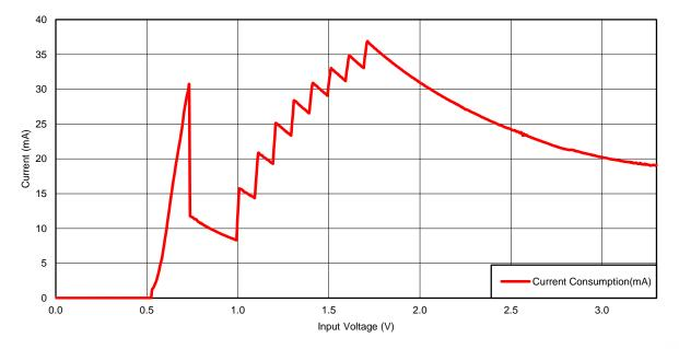
Figure 9. Total Current Consumption Versus Input Voltage
