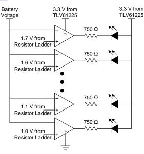
Figure 2. LM339 Application Schematic
