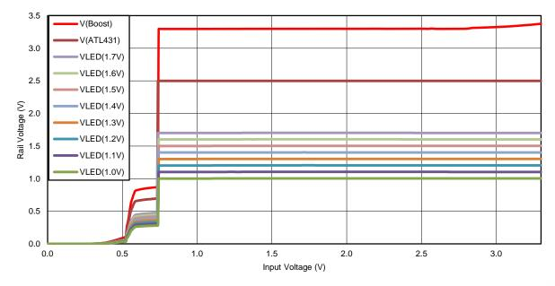
Figure 10. Device Voltage Rails Versus Input Voltage
