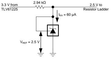
Figure 1. ATL431 Application Schematic
