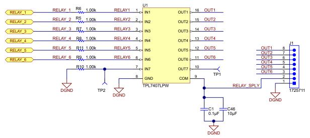
Figure 14. Digital Output Driver Circuit
