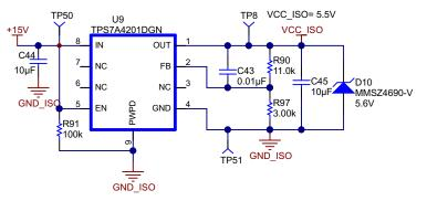
Figure 20. Regulator for DAC 5.5 V
