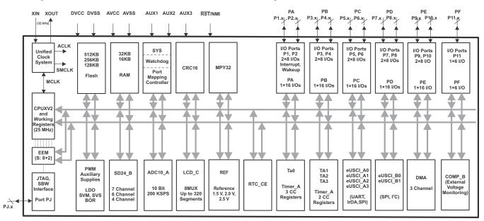
Figure 4. MSP430F67791A Functional Block Diagram
