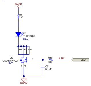
Figure 17. LED Driver Schematic
