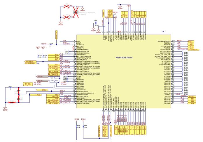
Figure 15. MSP430F67791A MCU Hardware Configuration Schematics
