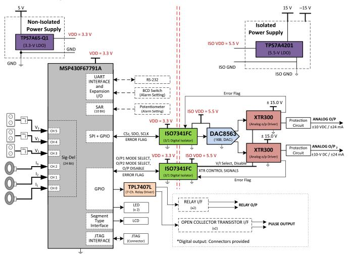
Figure 1. TIDA-00454 Functional Block Diagram
