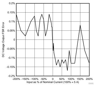
Figure 36. DC Voltage Output Accuracy Test for AOUT0
