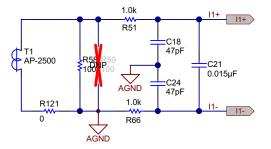
Figure 9. Circuit Diagram of Current Input
