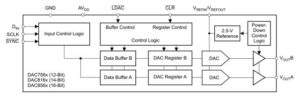
Figure 2. DAC856x Functional Block Diagram
