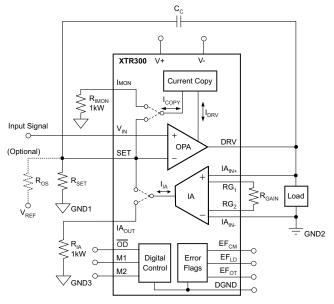
Figure 3. XTR300 Functional Block Diagram
