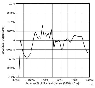
Figure 34. DAC8563 Output Accuracy Test
