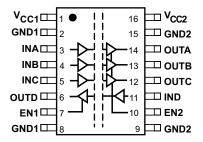
Figure 5. ISO7341FC Pin Configuration and Function
