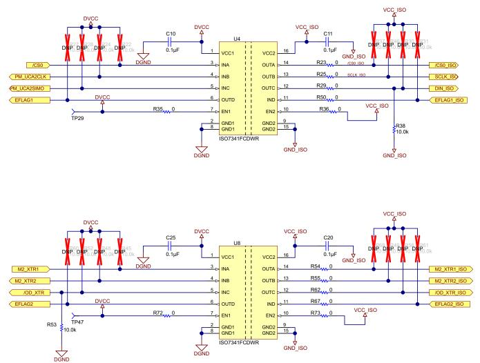
Figure 13. Circuit Diagram of Digital Isolators Interface
