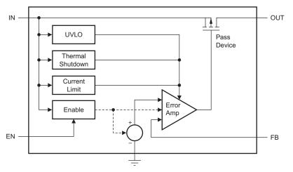
Figure 7. TPS7A42 Functional Block Diagram
