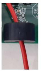
Figure 22. Current Input Wire Through CT
