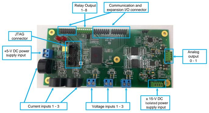
Figure 23. TIDA-00454 Interface Connectors
