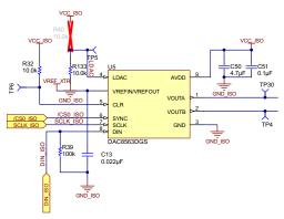
Figure 11. DAC8563 Circuit Diagram
