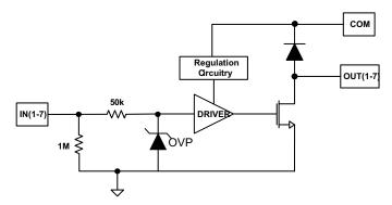
Figure 6. TPL7407L Functional Block Diagram
