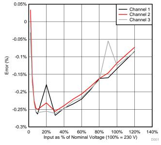
Figure 32. AC Input Voltage Accuracy Test
