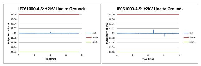
Figure 21: ±2 kV Surge - Line-to-Ground on I<sub>OUT</sub> (left) and RTN (right)
