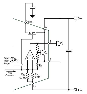
Figure 5: XTR105 Current Loop Transmitter Circuitry
