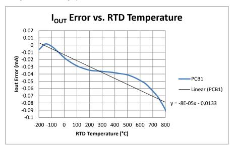
Figure 10: Output Current Error vs. RTD Temperature
