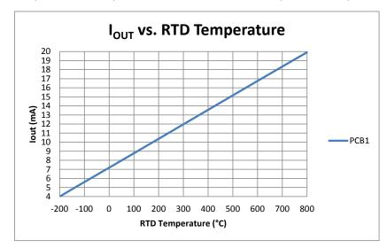
Figure 9: Output Current (I<sub>OUT</sub>) vs. RTD Temperature
