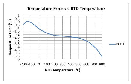
Figure 11: Output Temperature Error vs. RTD Temperature
