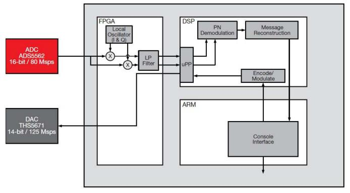
Figure 1. System Block Diagram for FPGA / DSP /ARM
