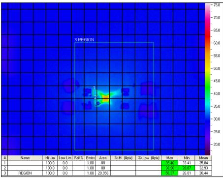
Figure 16 Thermal Camera Capture of LP5907UVX-3.3
