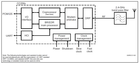
Figure 2 CC256X Functional Block Diagram
