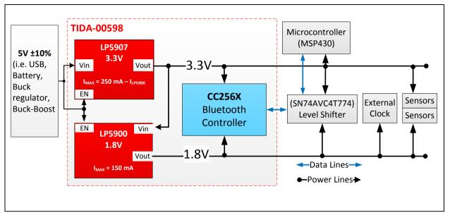
Figure 1 High Level Block Diagram of TIDA-00598 and Companion Devices
