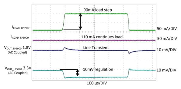
Figure 7: Load and Line Transients and Regulation of TIDA-00598
