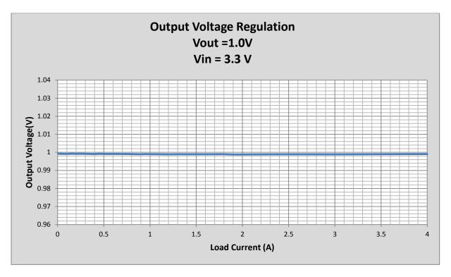
Figure 7 Output voltage vs Load Current
