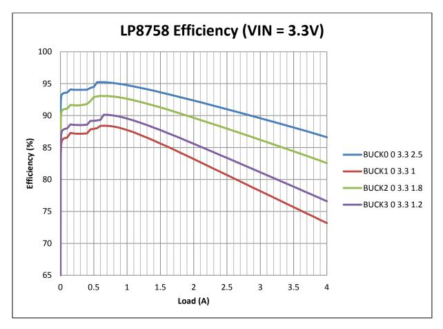
Figure 4: Output Voltage Efficiency in Auto Mode
