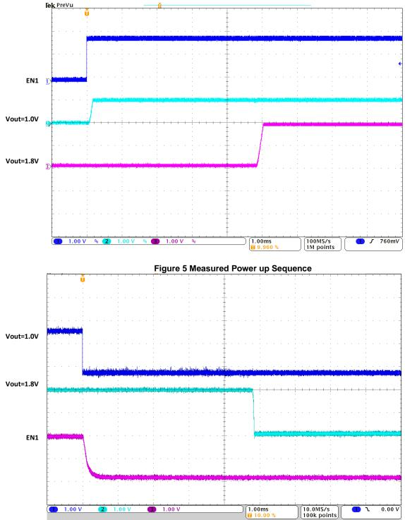
Figure 6 Measured Power down Sequence
