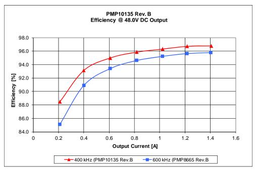
**Figure 3** *PMP8665RevB is modified to Vout 31V / Fsw 600kHz, PMP10135RevB chops at 400kHz*
