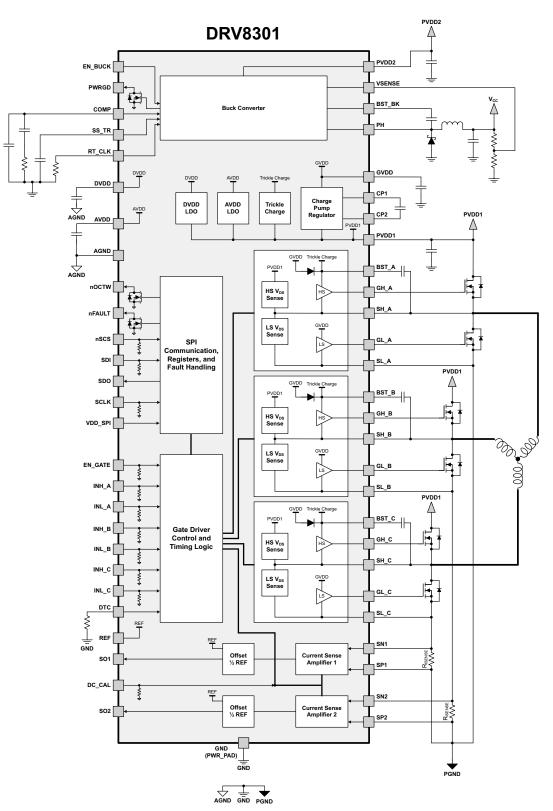
Figure 3. DRV8301 Three-Phase Gate Driver Functional Block Diagram
