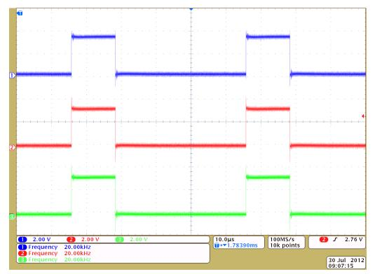
Figure 11. PWM Output on Pins 25, 26, and 28 of Connector J5
