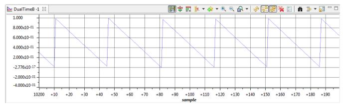
Figure 19. Encoder-based Electrical Angle
