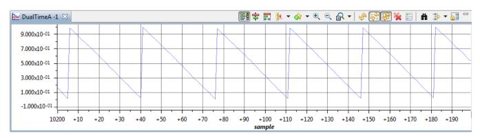
Figure 18. SMO-based Electrical Angle
