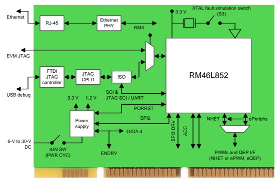
Figure 9. RM46x MCU Interfaces on the Control Card
