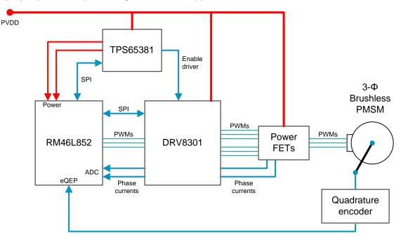
Figure 4. 3-Phase Brushless Permanent Magnet Synchronous Motor Drive Implementation
