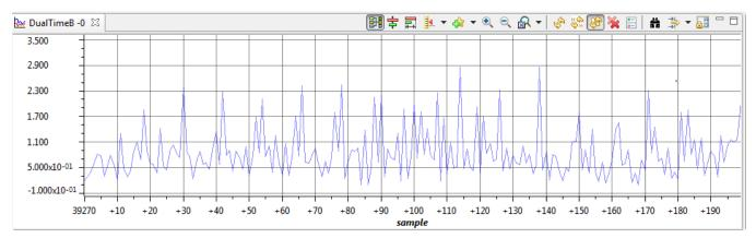
Figure 13. Total Motor Current
