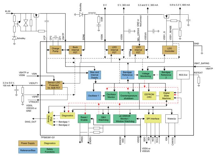
Figure 2. TPS65381 Functional Block Diagram
