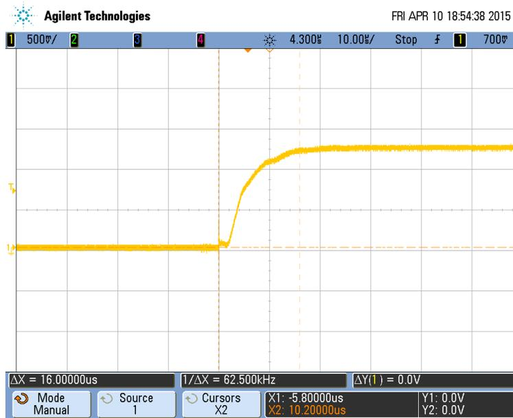
Figure 11. Start-Up Output Voltage Transient
