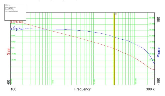
Output power = 1.3V@3.0AInput voltage = 5VDCPhase margin =  $59^{\circ}$ Bandwidth = 32.2kHz
