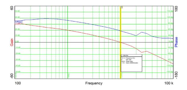
The plot below shows the loop gain with the input voltage set to 24V and for an output load of 10A.
