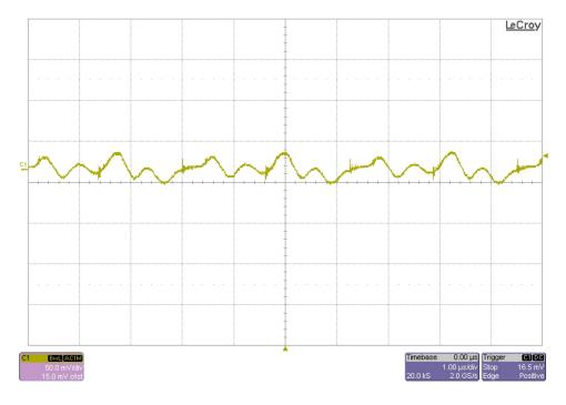
The 15V output ripple voltage (AC coupled) is shown in the figure below. The image was taken with the output loaded to 10A. The input voltage is set to 24V. (50mV/DIV, 1uS/DIV)
