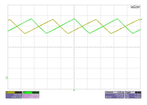
The photo below shows the measured inductor current in each phase. The input voltage was set to 24V with a 10A load. (2A/DIV, 1uS/DIV)
