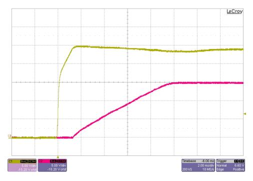
The photo below shows the output voltage startup waveform after the application of 24V in. The 15V output was loaded to 20A. (5V/DIV, 2mS/DIV)
