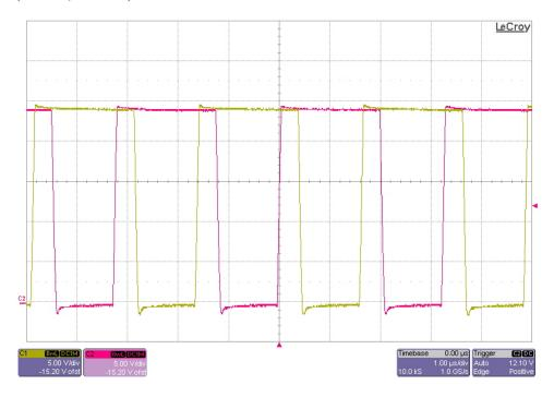
The photo below shows the FET switching voltages of each phase for an input voltage of 24V and a 20A load. (5V/DIV, 1uS/DIV)
