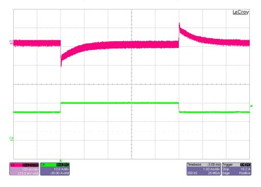
The photo below shows the 15V output voltage (ac coupled) when the load current is stepped between 10A and 20A. Vin = 24V. (200mV/DIV, 10A/DIV, 1mS/DIV)
