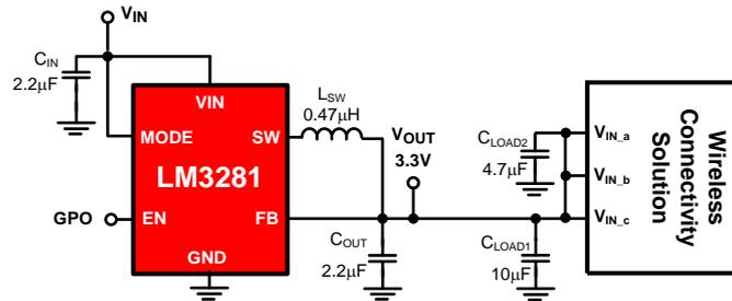
Figure 7 Application schematic
