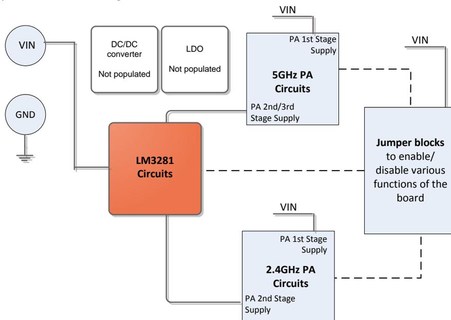
**Figure 1** TIDA-00532 design high level block diagram
