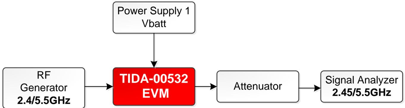
Figure 8 Test Setup Block Diagram
