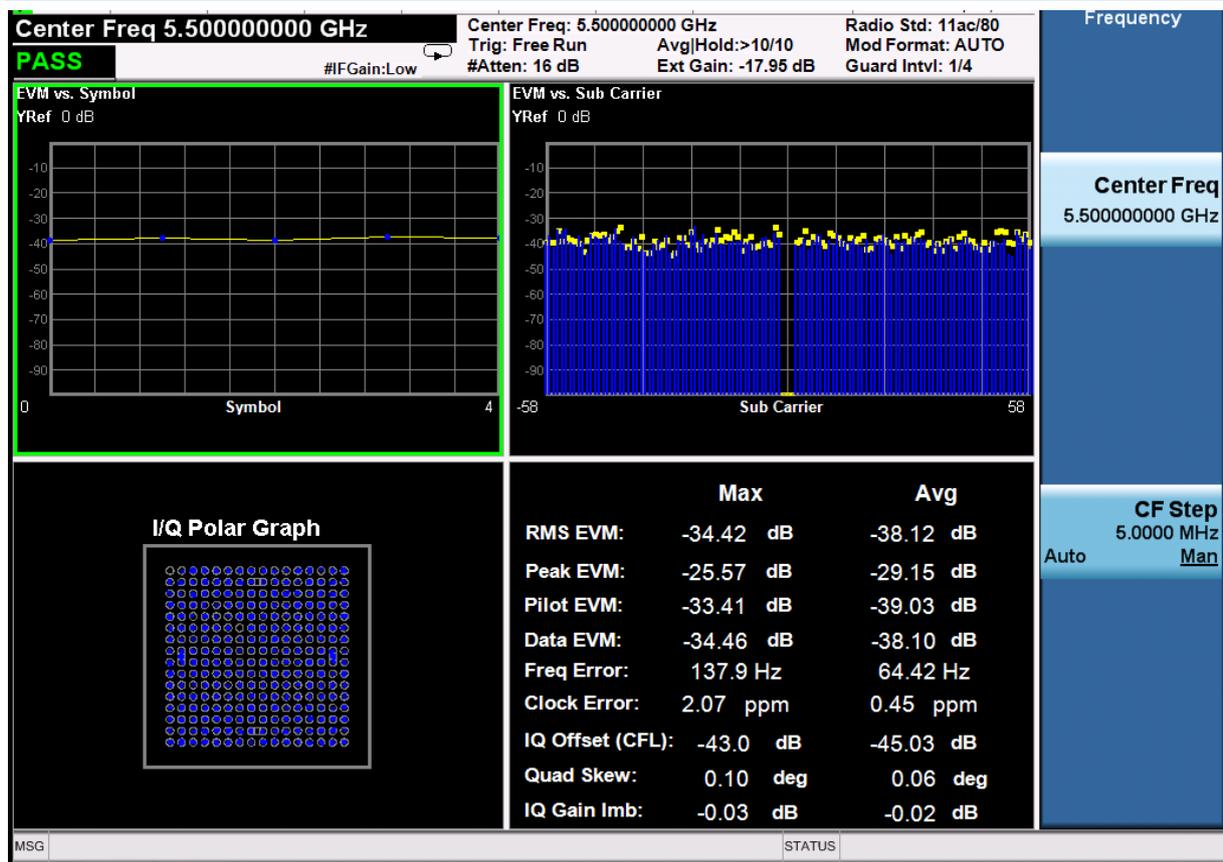
Figure 9 EVM measurements with LM3281 and TQP887051 5GHz FEM
