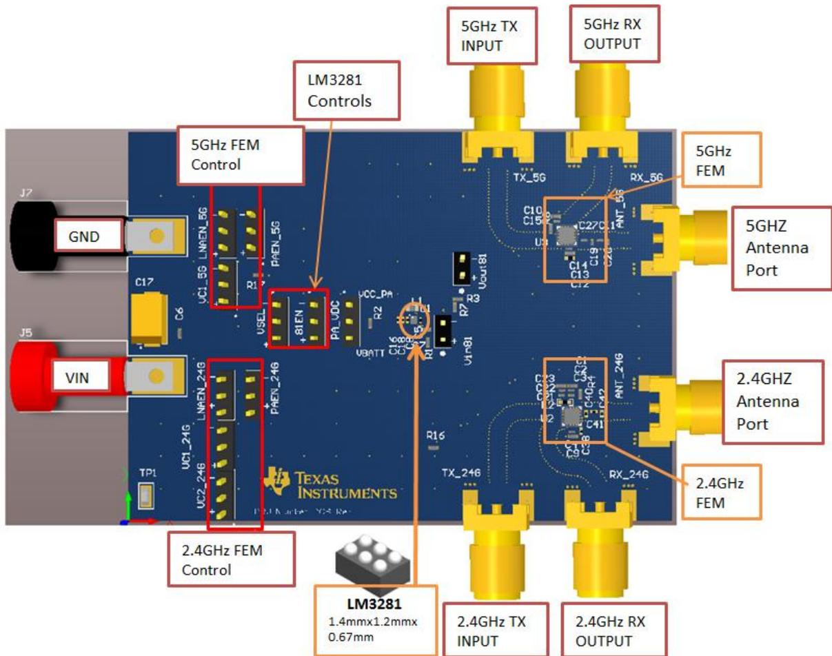
Figure 2 3D view of TIDA-00532 EVM with major connectors and components identified.
