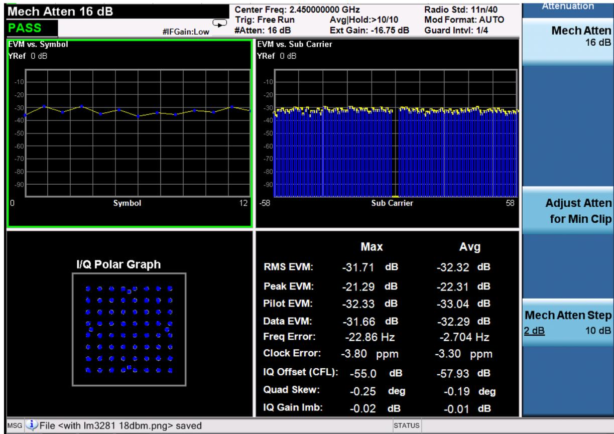
Figure 13 EVM measurements with direct connection to VBATT using TQF9046 2.4GHz FEM
