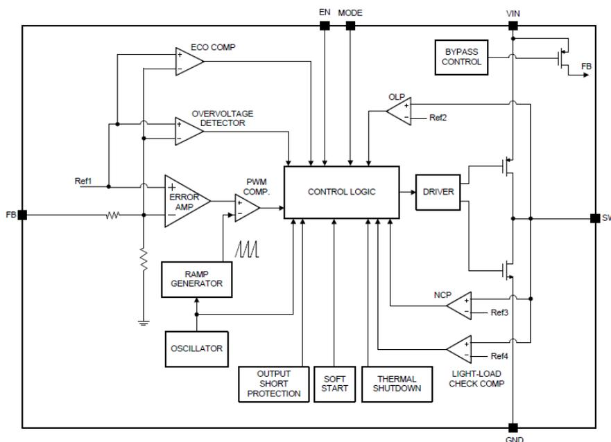
**Figure 4 LM3281 functional block diagram**
