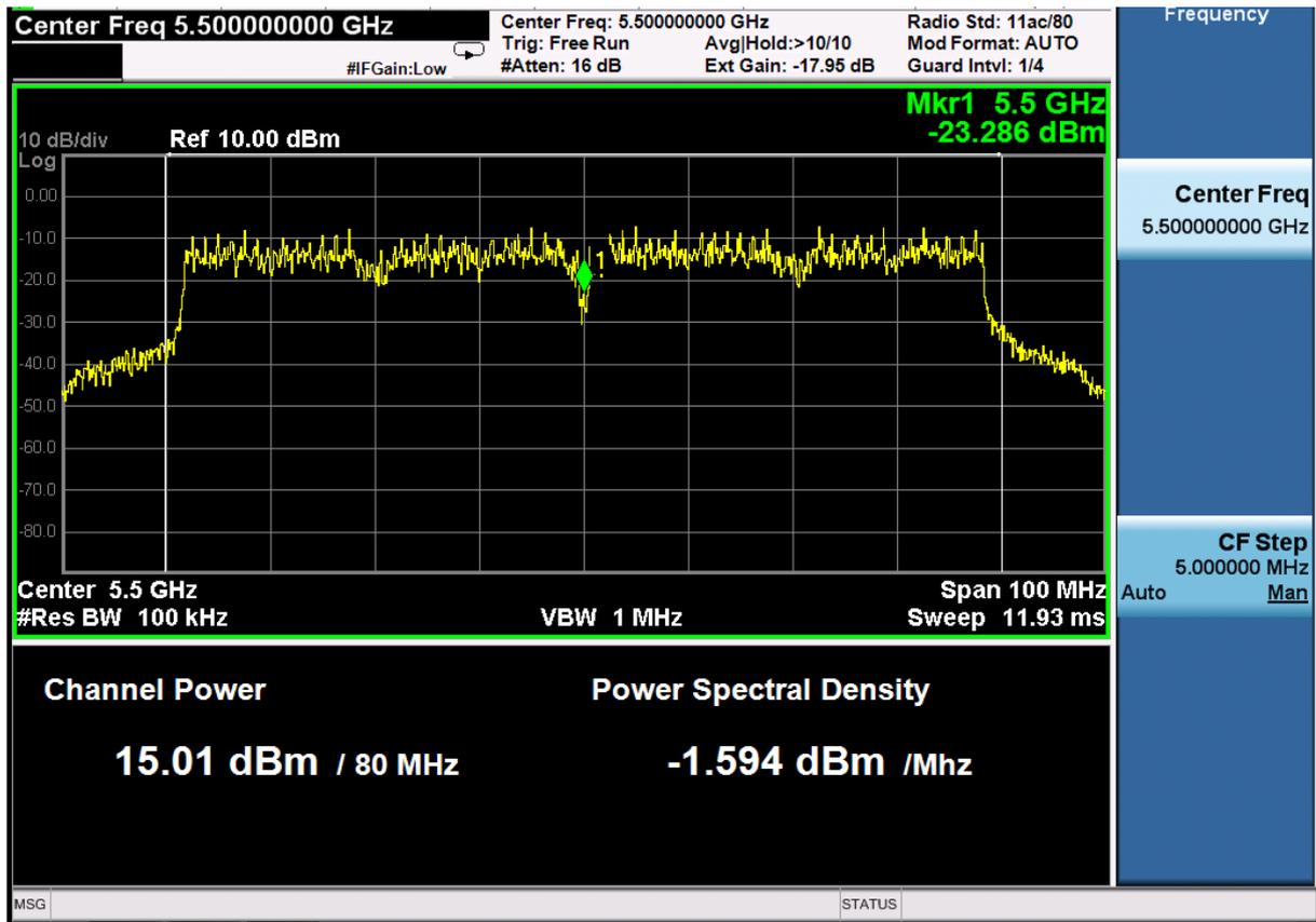
Figure 11 Channel Power measurements with LM3281 and TQP887051 5GHz FEM
