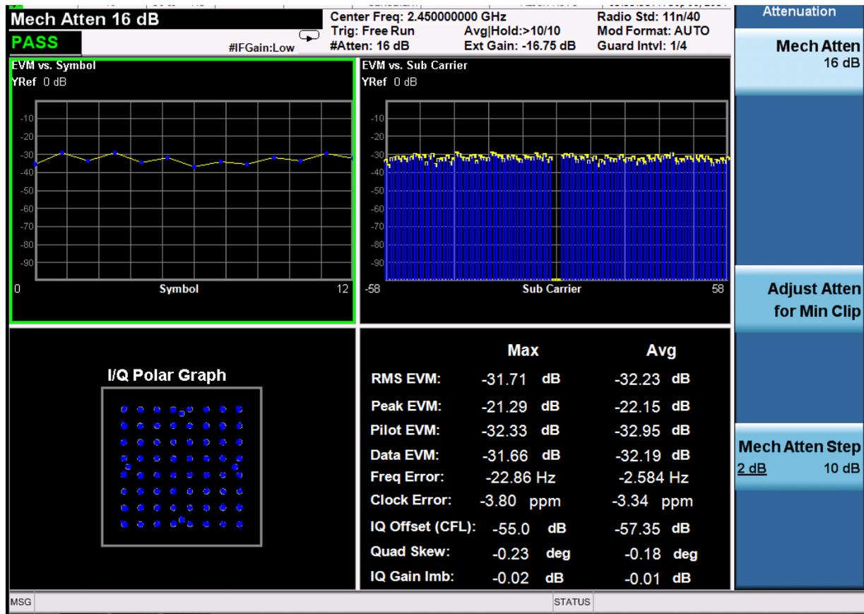
Figure 12 EVM measurements with LM3281 and TQF9046 2.4GHz FEM
