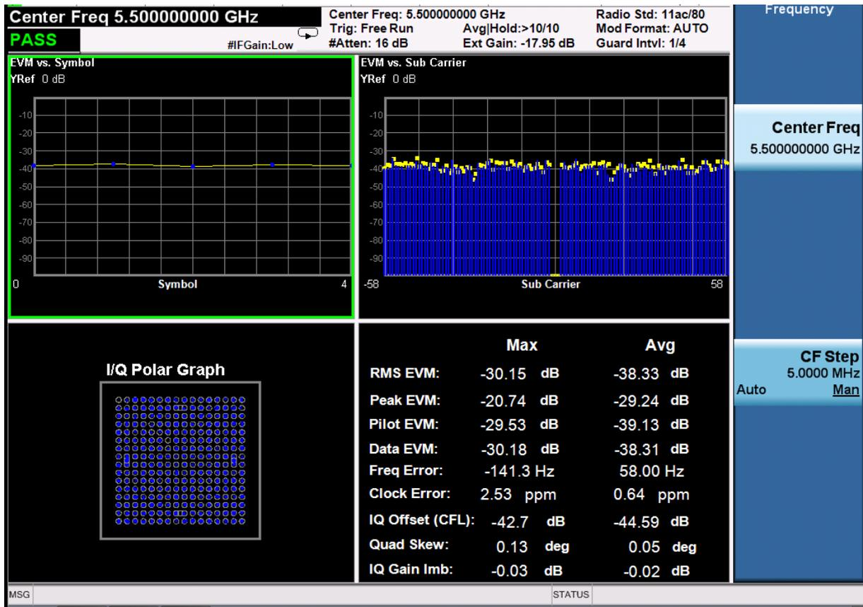
Figure 10 EVM measurements with direct connection to VBATT using TQP887051 5GHz FEM
