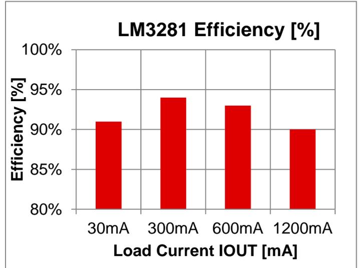
Figure 6 LM3281 Efficiency
