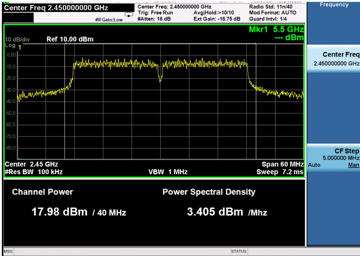
Figure 14 Channel Power measurements with LM3281 and TQF9046 2.4GHz FEM
