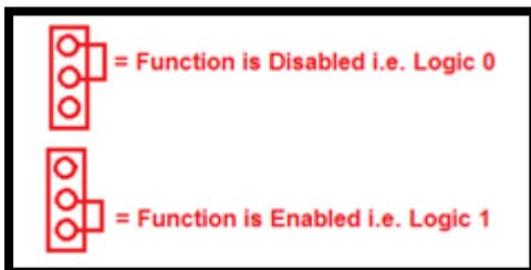
Figure 3 Three Pin Header Legend
