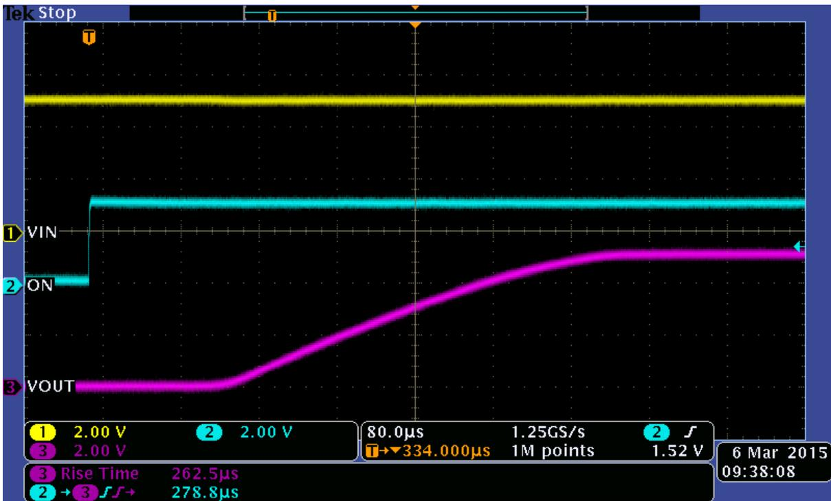
Figure 8. Dual TPS22966 Turn On Waveform with  $V_{IN} = V_{BIAS} = 5\text{ V}$
