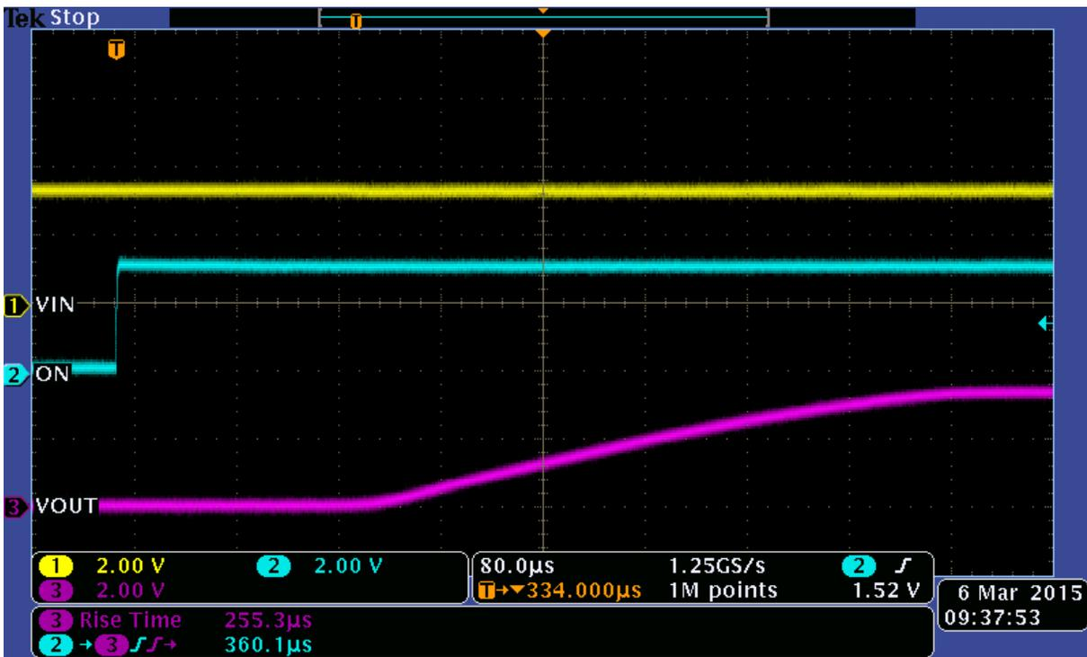
Figure 7. Dual TPS22966 Turn On Waveform with  $V_{IN} = V_{BIAS} = 3.3\text{ V}$
