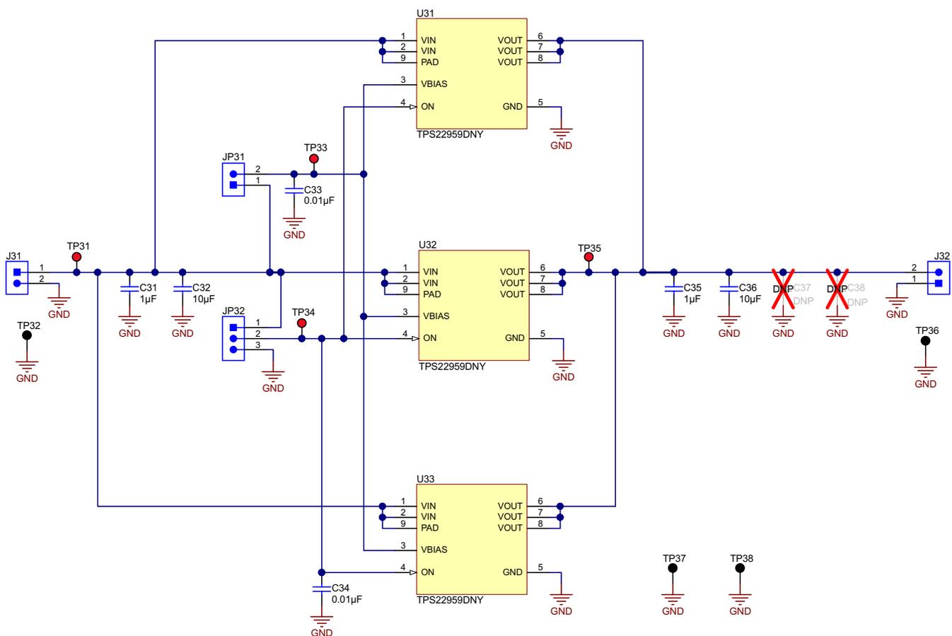
Figure 12. Triple TPS22959 Schematic
