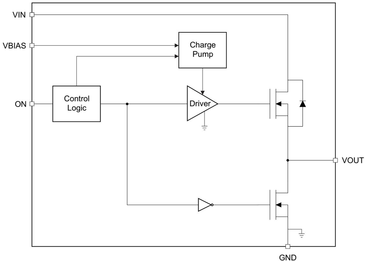
**Figure 4. TPS22959 Functional Block Diagram**
