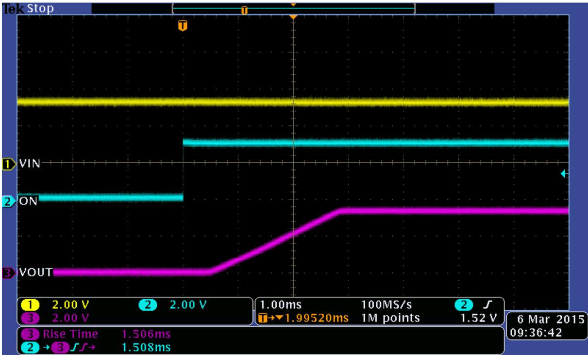
Figure 9. Triple TPS22959 Turn On Waveform with  $V_{IN} = V_{BIAS} = 3.3\text{ V}$
