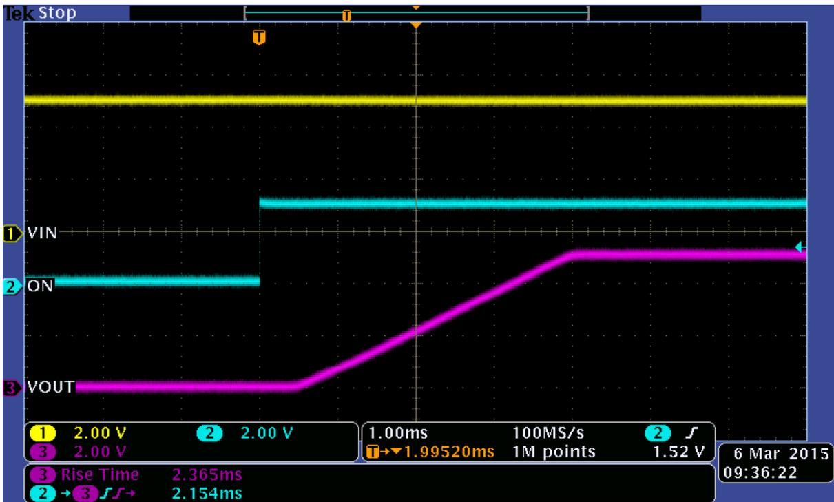
Figure 10. Triple TPS22959 Turn On Waveform with  $V_{IN} = V_{BIAS} = 5\text{ V}$
