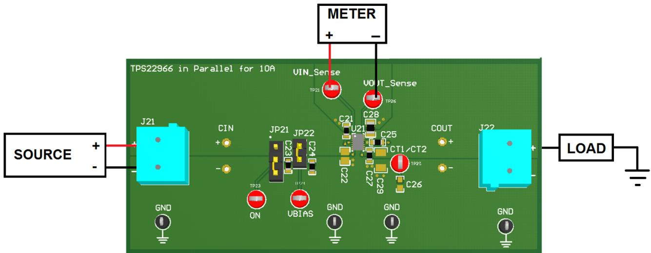
Figure 5. ON Resistance Test Setup
