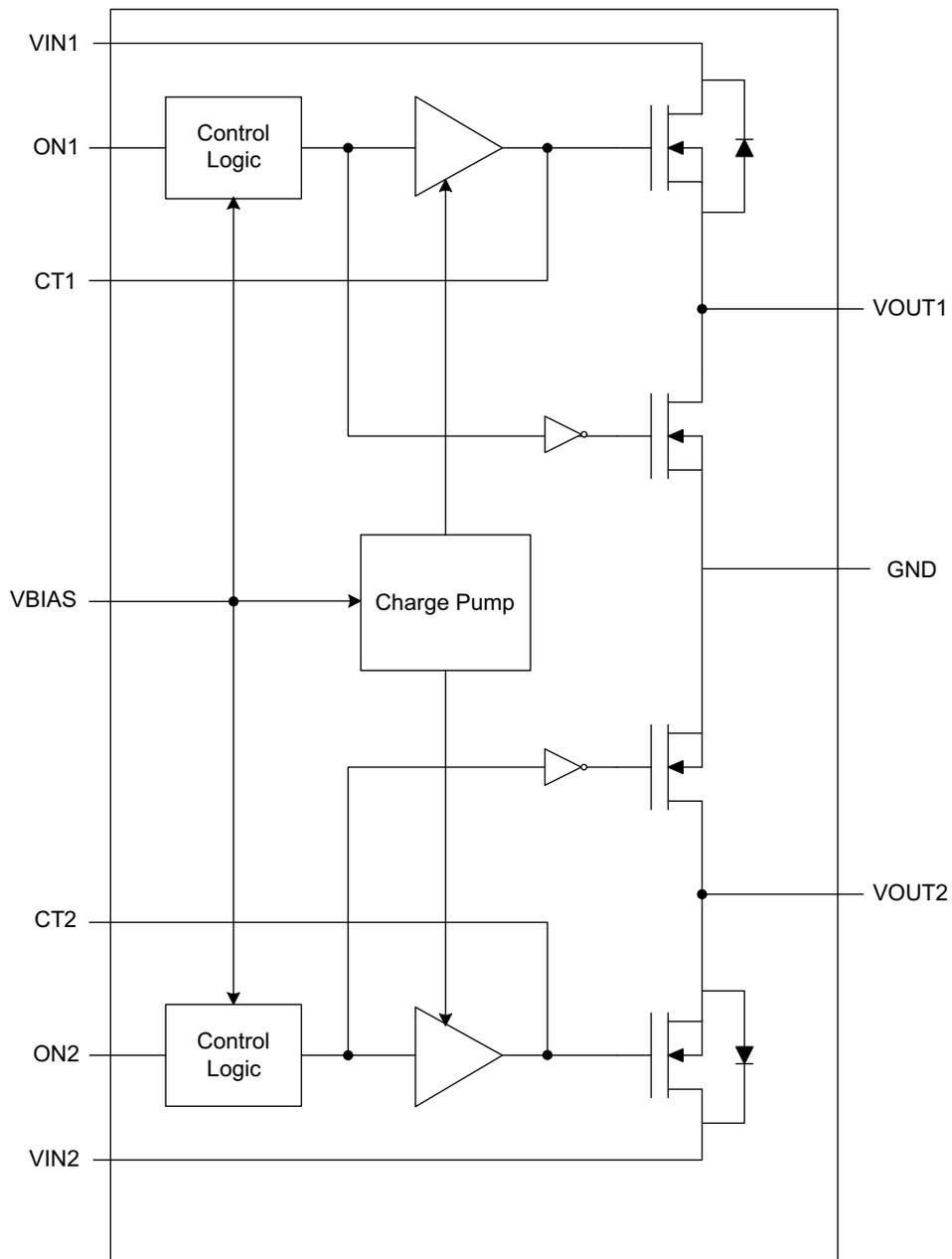
Figure 3. TPS22966 Functional Block Diagram
