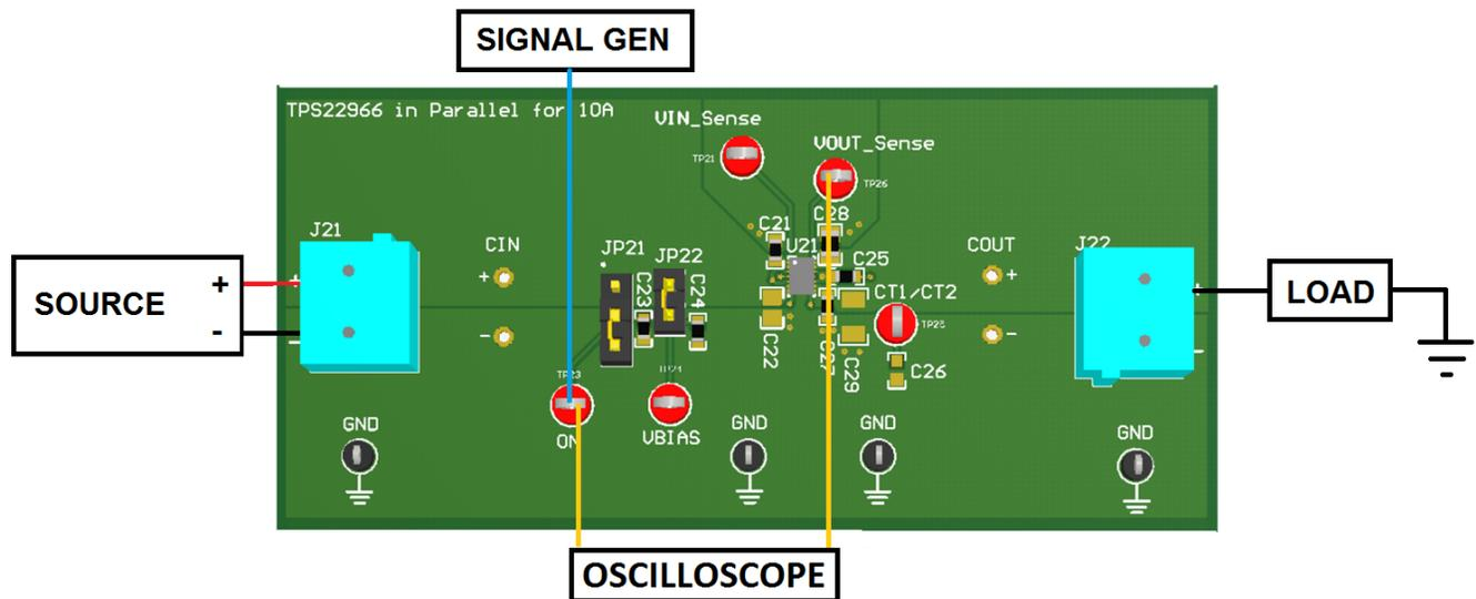
Figure 6. Turn On Test Setup
