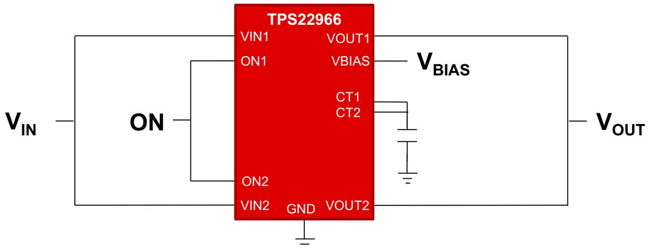
Figure 1. Dual TPS22966 Block Diagram
