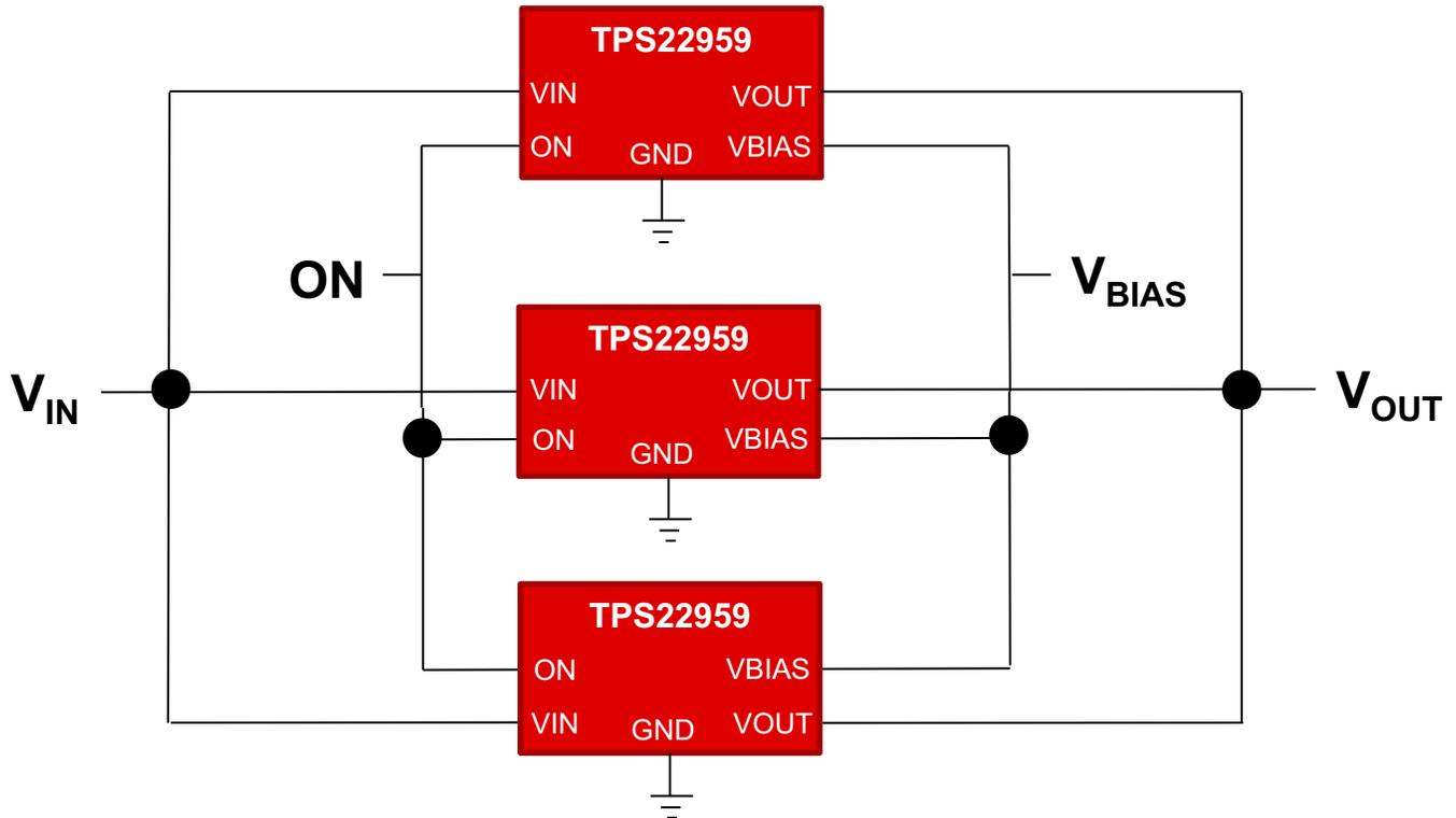
Figure 2. Triple TPS22959 Block Diagram
