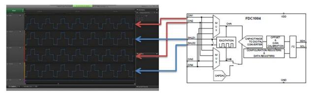
If the capacitance of the shield is too large, it can have negative impacts on the measured capacitive values. For comparison, below is a demonstration of a shield driver that is saturated due to a larger than acceptable shield capacitance.
