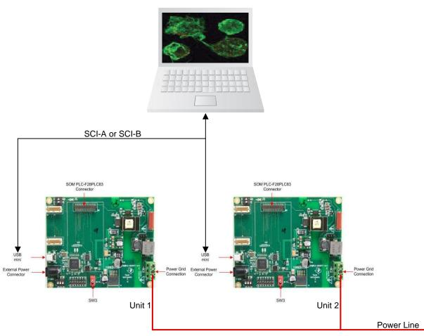
Figure 9. Testing Setup
