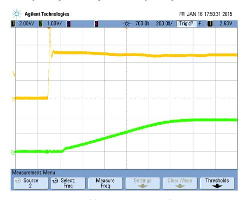
Figure 5 Start up into no load at 5Vin
