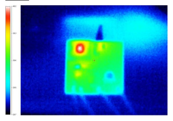
IR Thermal Image taken after running at 12V in, 1A load running for 15 Minutes; Room Temp = 24.5C
