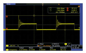
Primary-Side Switch Voltage at 12Vin and 1Aout (Energy spike does exceed the max VDS rating of MOSFET (40V)) – Recommend Infineon, BSZ042N06 as a direct higher voltage replacement. Another alternative for possible improvement in efficiency in the Infineon, BSZ067N06.
