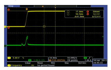
Startup into No Load (12Vin)
