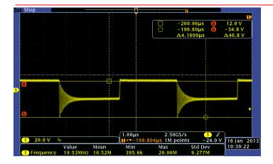
Secondary-Side Switch Node at 12Vin 1A load (ringing is exceeding max VRRM of diode (40V)) Recommend On Semi, MBRD350 as a suitable replacement.
