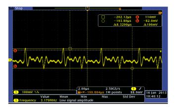
Output Voltage Ripple 12V in 1A out.
