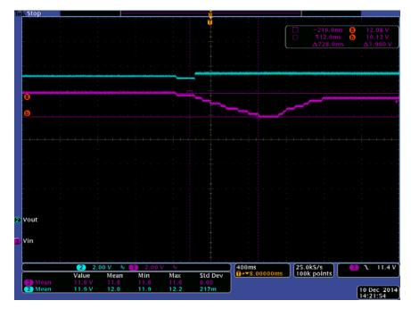
Figure 18. Bypass to Boost Transition with 33A Load (Channel 2 = VOUT, Channel 3 = VIN)
