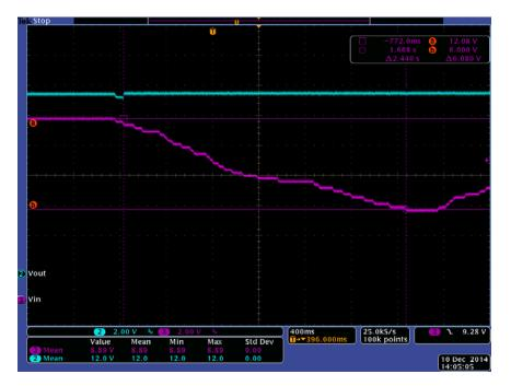
Figure 7. Bypass to Boost Transition with 5A Load (Channel 2 = VOUT, Channel 3 = VIN)
