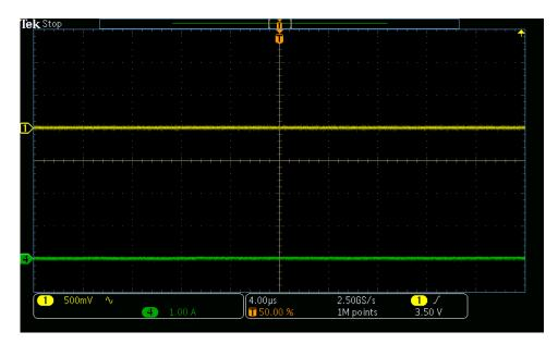
Figure 26. AC Coupled Output Voltage Ripple with No Load (VIN = 12V, Channel 1 = VOUT, Channel 4 = IOUT)
