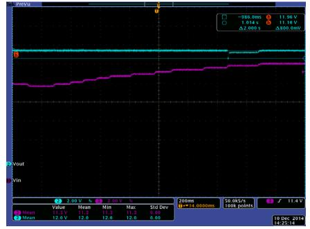
Figure 22. Boost to Bypass Transition with 30A Load (Channel 2 = VOUT, Channel 3 = VIN)
