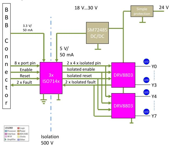
Figure 1. TIDA-00320 Block Diagram
