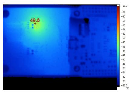
Figure 9. Thermal Scan of PCB Bottom Under Load
