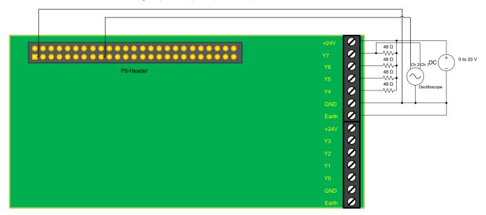
Figure 6. Measurement Setup for Rise, Fall, and Propagation Delay Times
