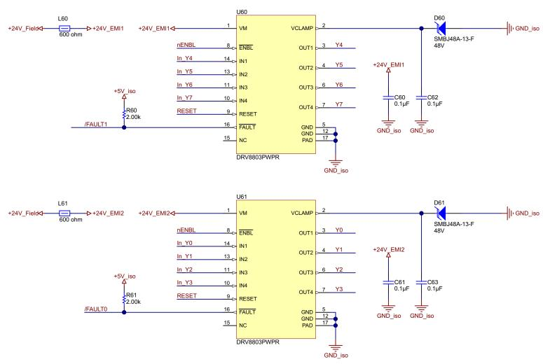
Figure 16. Digital Output Stage
