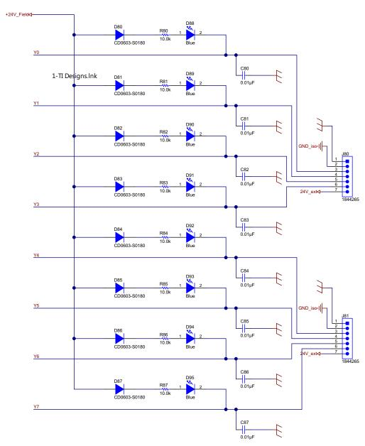
Figure 17. Output Connectors and Surge Protection1
