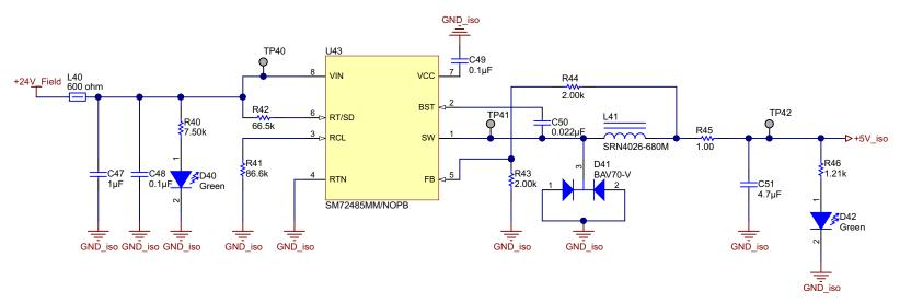
Figure 15. Digital Isolators and Field Power Supply2
