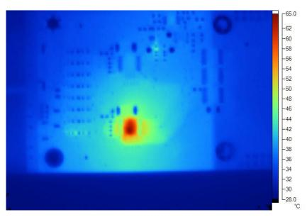
Figure 10. Thermal Scan of PCB Top Under Load
