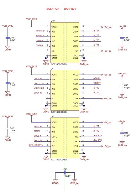
Figure 14. Digital Isolators and Field Power Supply1
