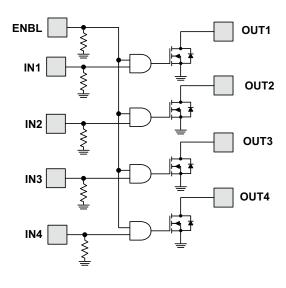
Figure 2. DRV8803 Block Diagram
