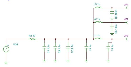
Figure 4. EMI Filter Simulation Model
