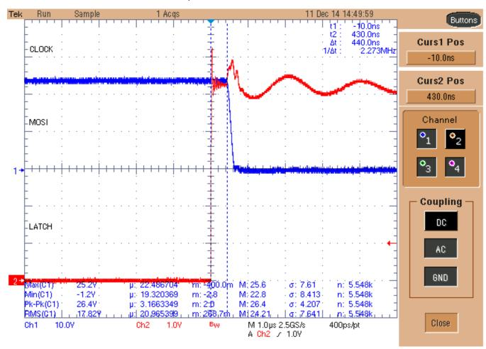
Figure 7. Fall Time and Propagation Delay
