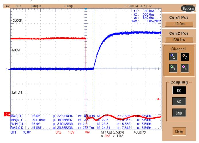
Figure 8. Rise Time and Propagation Delay
