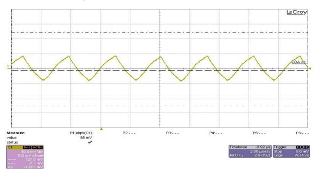
Test condition: The input voltage was set at 24V, and four outputs were set at full load of 75mA. Ch1 - 5VP (+5V) (AC coupled)
