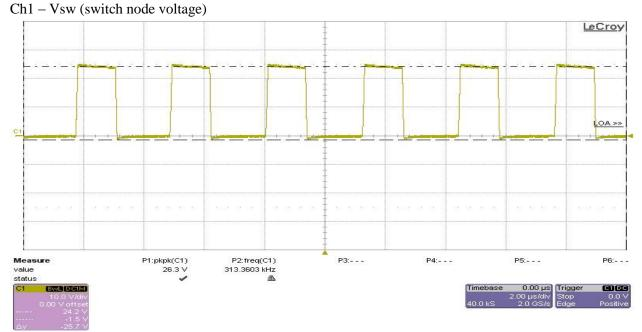
Test condition: The input voltage was set at 32V, and four outputs were set at full load of 75mA.
