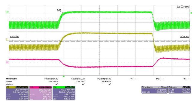
Test condition: Vin = 24V, 5VP (+5V) load from 0A to 75mA, no load at the other outputs. Ch1- 5VP (+5V) (AC mode), Ch2- 5VN (-5V) (AC mode), Ch4- Io (+5V output current)
