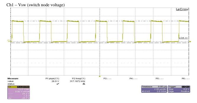
Test condition: The input voltage was set at 24V, and four outputs were set at full load.
