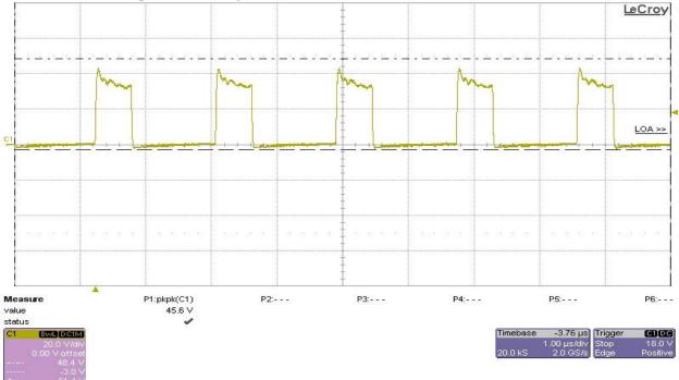
Ch1 – Vd12 (12V output diode voltage stress from cathode (-) to anode (+))
