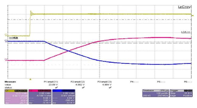
Test condition: The input voltage was set at 24V, and both outputs were set at full load of 75mA. Ch1 - Vin, Ch2 - 5VP (+5V), Ch3 - 5VN (-5V)
