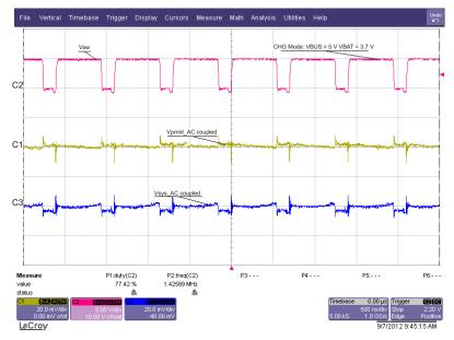
Figure 4. CHG Mode Ripple and Duty Cycle: V<sub>BUS</sub> = 5 V, V<sub>BAT</sub> = 3.7 V
