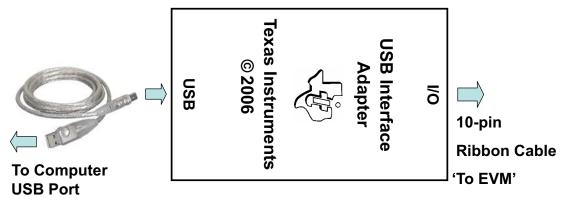
Figure 1. Connections of the HPA172 Kit
