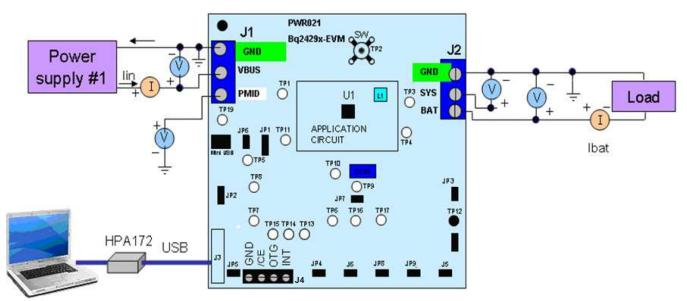
Figure 2. Original Test Setup for PWR021 (bq2429xEVM)
