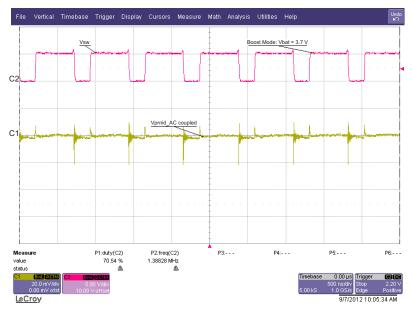
Figure 5. Boost Mode Ripple and Duty Cycle; V<sub>BAT</sub> = 3.7 V
