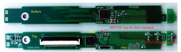
Figure 5. Debug and Programming Interface
