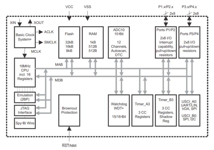
Figure 1. Functional Block Diagram, MSP430G2x44
