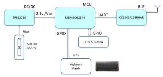
Figure 3. Hardware Block Diagram
