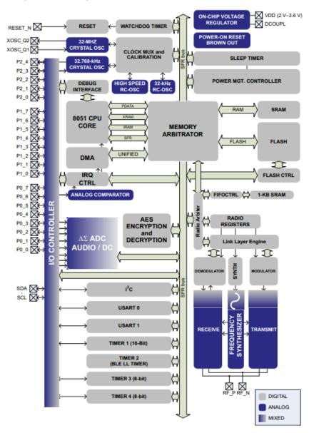
Figure 2. CC2541 Simplified Block Diagram
