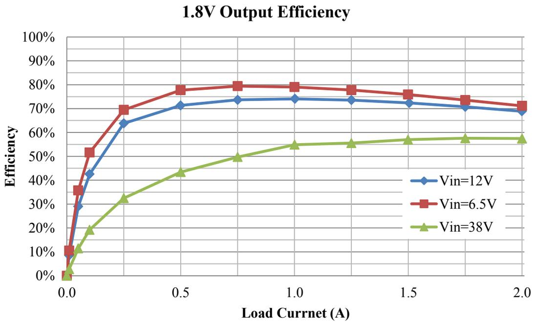
Figure 7 1.8V Output Efficiency
