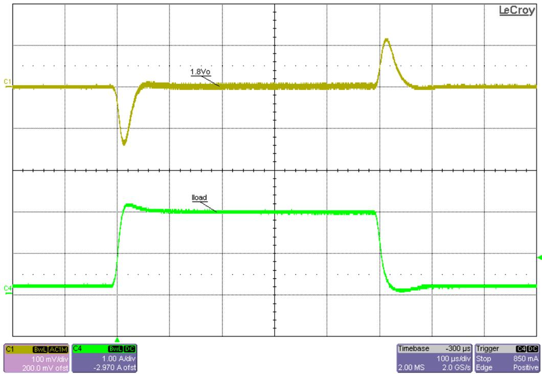
Figure 19 1.8V Output Buck Regulator Load Transient
