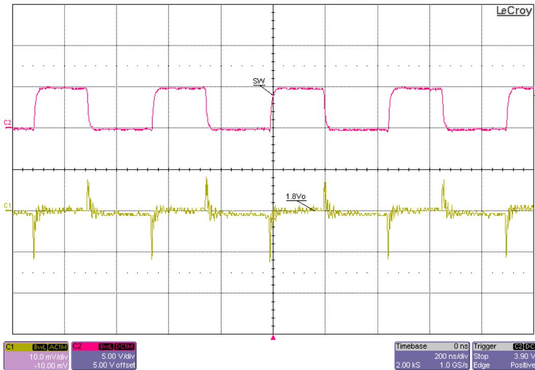
Figure 22 1.8V Output Ripple at 2A Load
