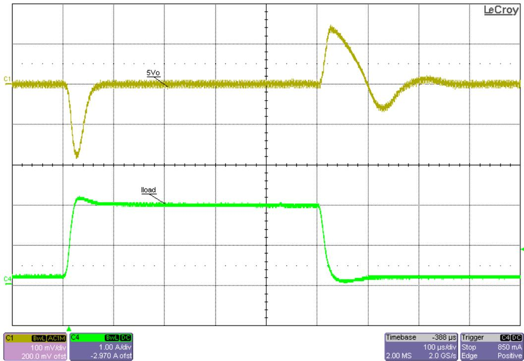
Figure 17 5V Output Buck Regulator Load Transient
