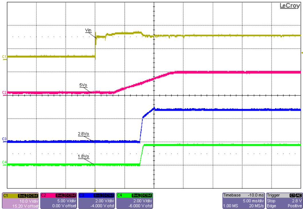
Figure 15 Power Up into Full Load at 12Vin
