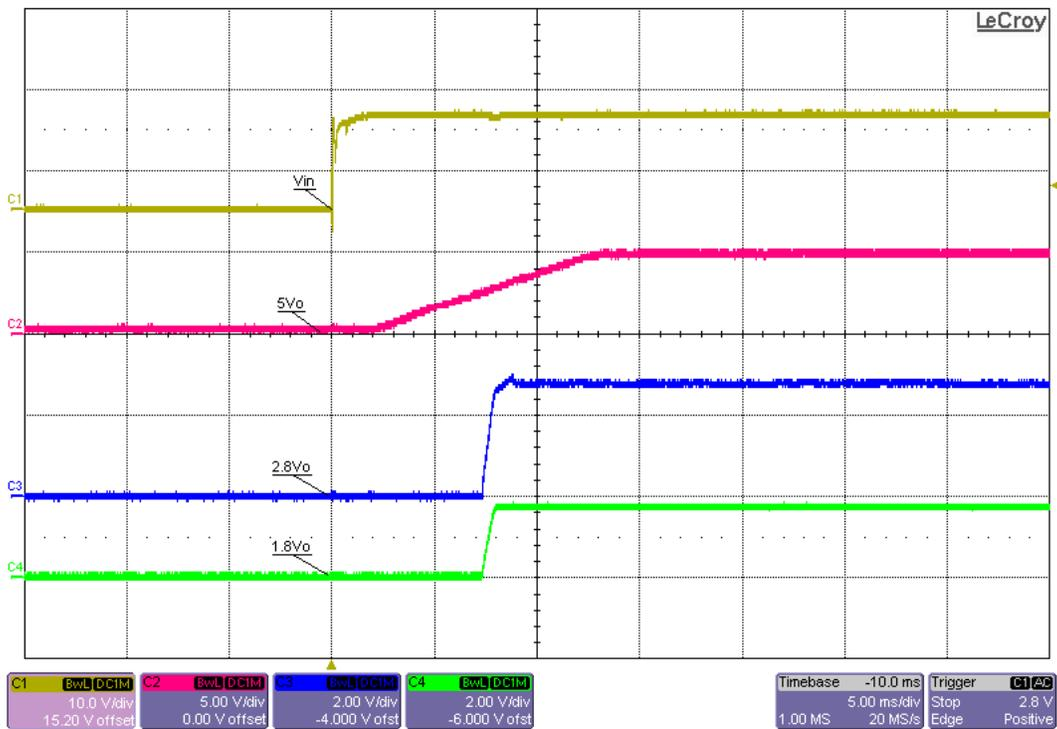
Figure 16 Power Up into No Load at 12Vin
