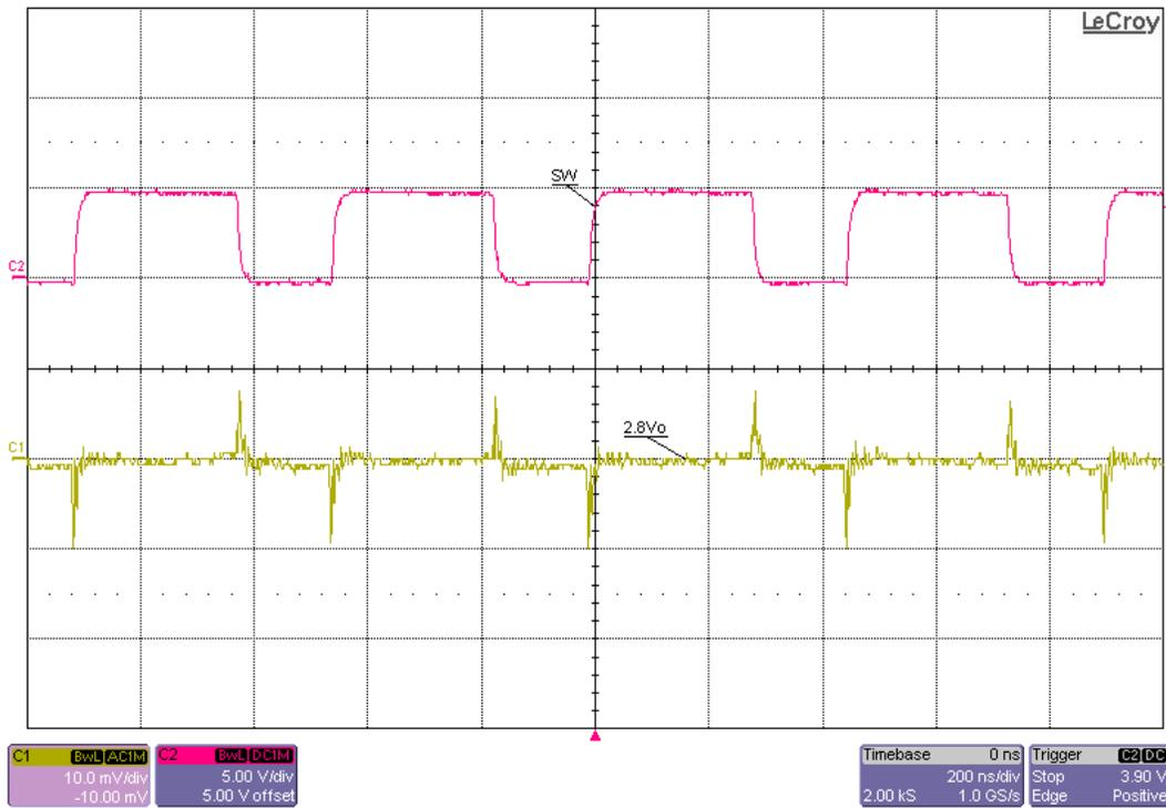
Figure 21 2.8V Output Ripple at 1.5A Load
