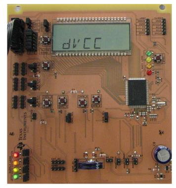
Figure 6. AUX01 Code Example: Chip Powered from DVCC
