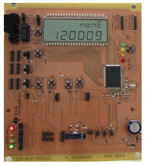
Figure 24. AUX15 Code Example: Initial Condition, No Tamper Event
