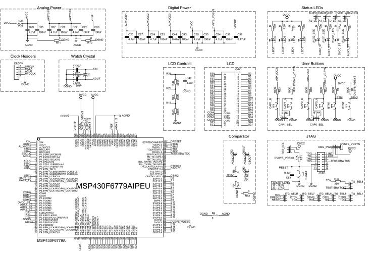
Figure 30. TIDM-AUX-MODULE Schematic Page 1
