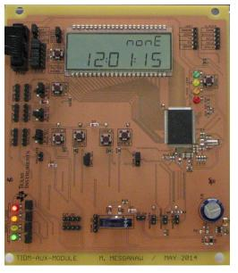
Figure 18. AUX14 Code Example: Initial Condition, No Tamper Event
