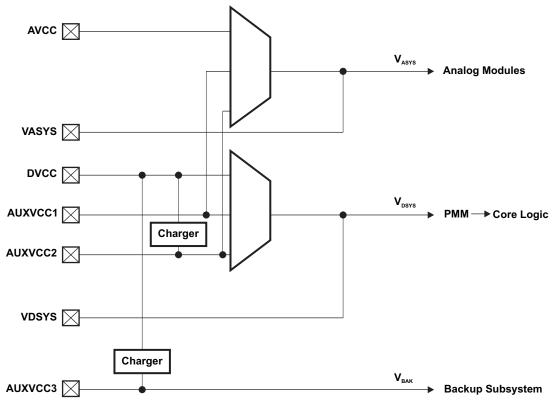
Figure 1. AUX Module Functional Block Diagram
