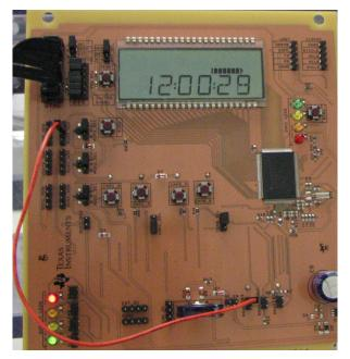
Figure 13. AUX07 Code Example: AUXVCC3 Voltage Rises Above 2.5-V Threshold After Falling Below It
