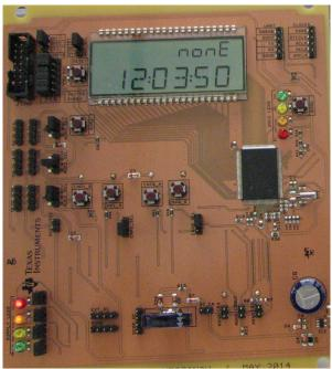
By pressing BTN2, the RTC event is cleared, which is shown in Figure 22.
