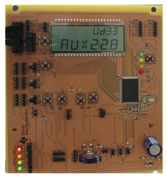
Figure 14. AUX10 Code Example: AUXVCC2 and VDSYS Voltage Measurement Results
