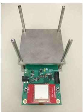
Figure 10. Mechanical Setup with Reference Design PCB and Top Plate
