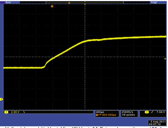
Yellow(channel 1)=Vout; Vin=48V lout=0A External capacitance=150uf
