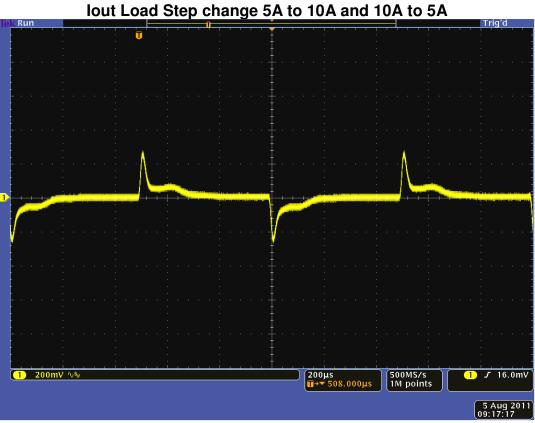
Vout response with 50% step change in load. External capacitance=150uf
