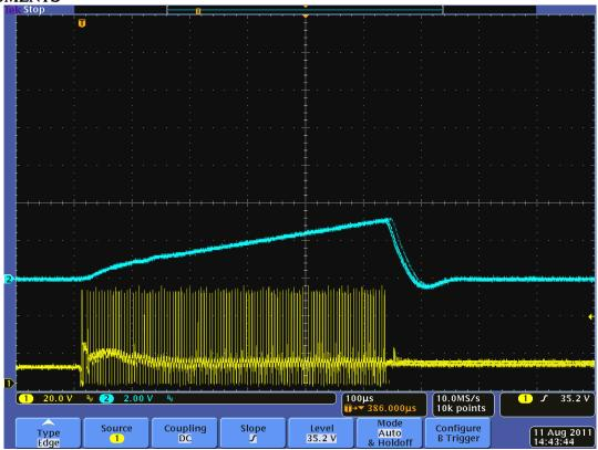
Yellow(channel 1)=Transformer Primary Voltage, Blue(channel 2)=Vout; lout=20A External capacitance=150uf
