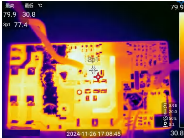
Figure 2-7. Thermal, 230VAC, Full Load
