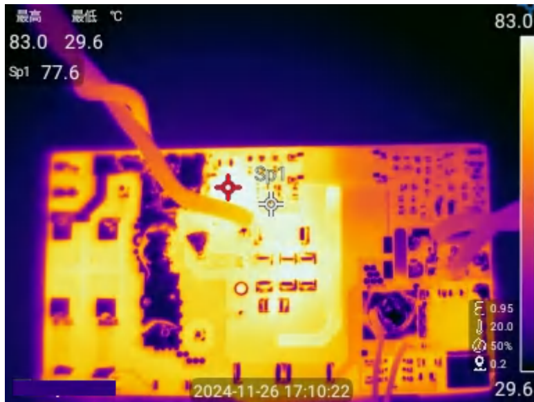
Figure 2-8. Thermal, 264VAC, Full Load
