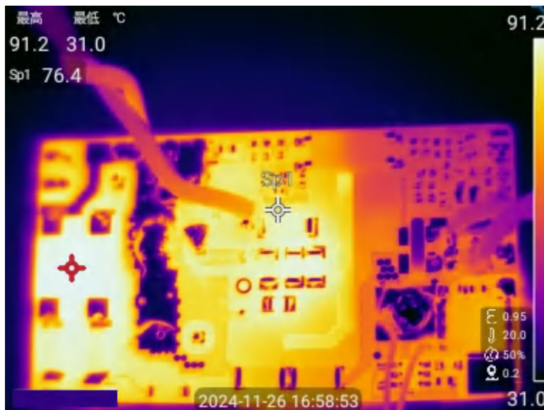
Figure 2-6. Thermal, 115VAC, Full Load
