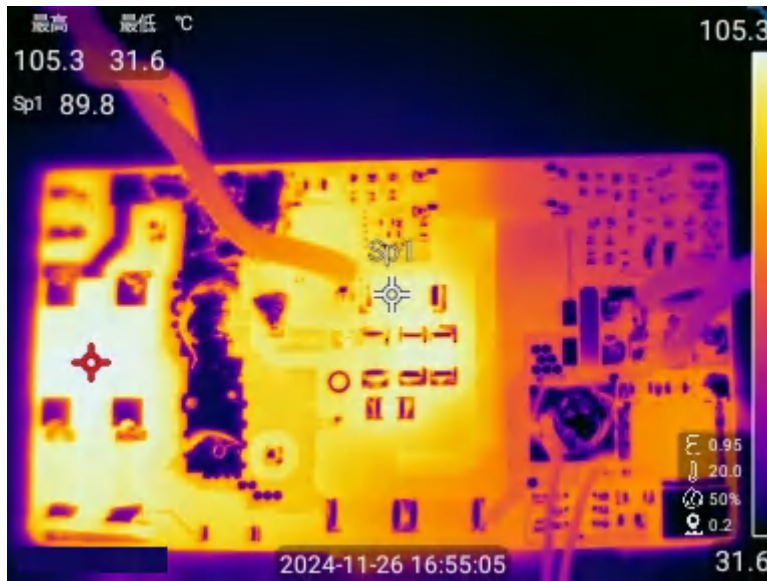
Figure 2-5. Thermal, 90VAC, Full Load
