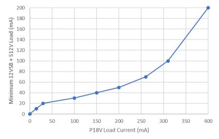
Figure 1-1. P18V Minimum Load Requirements
