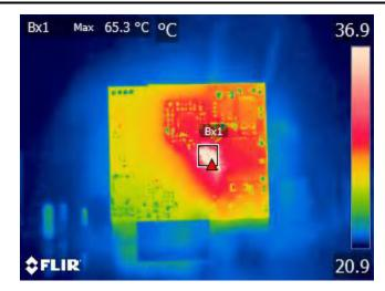
Figure 3-6. Thermal Image OFF State(GaN-Side of Assembly)
