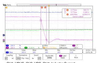
CH1: VBUS, CH3: VDS, CH4: Inductor Current Figure 3-7. Falling Edge Behavior of PFC Stage
