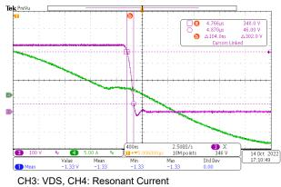
Figure 3-4. Falling Edge Behavior of LLC Stage
