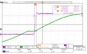
CH3: VDS, CH4: Resonant Current Figure 3-5. Rising Edge Behavior of LLC Stage
