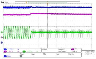
CH1: Output Voltage, CH3: VBUS, CH4: Input Current Figure 3-9. 50% Load to 0% Load
