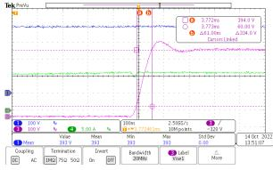
CH1: VBUS, CH3: VDS, CH4: Inductor Current Figure 3-6. Rising Edge Behavior of PFC Stage
