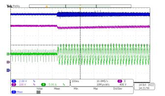
CH1: Output Voltage, CH3: VBUS, CH4: Input Current Figure 3-8. 0% Load to 50% Load
