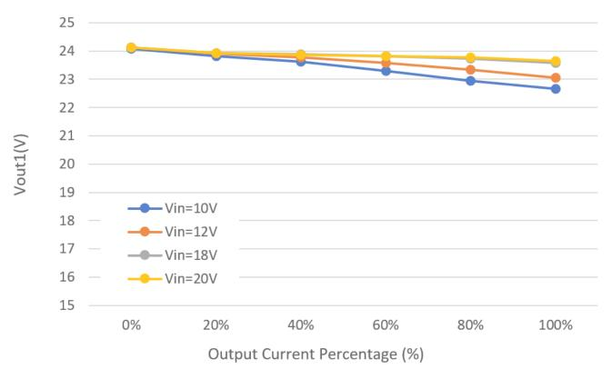
Figure 2-2. Isolated V<sub>OUT1</sub> and V<sub>OUT2</sub> Regulation With Same Percentage Current (Vout1)
