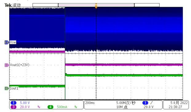
Figure 3-13. Output Short From Double Full-Load Operation To Short Circuit at 12-V Input (+23-V Rail Short Circuit)
