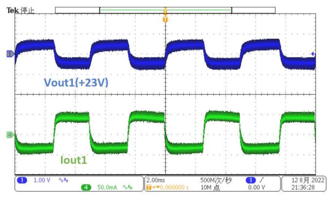
Figure 3-8. +23-V Output Load Transient at 12-V Input From 0 mA to 80 mA
