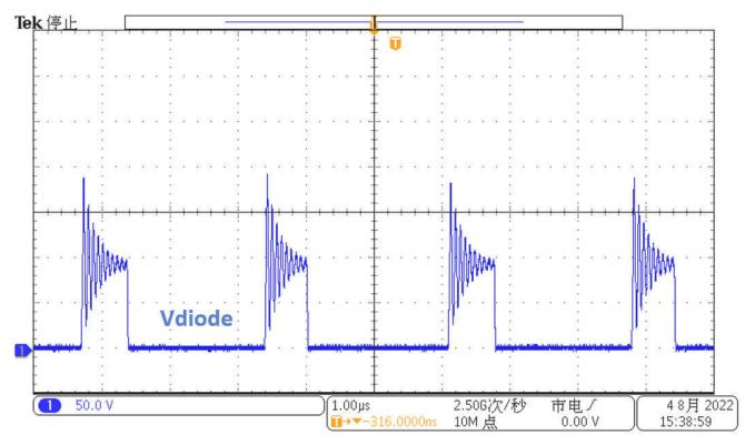
Figure 3-18. Channel A Diode Voltage Stress  $V_{IN}$  = 20 V,  $I_{OUT1}$  = 80 mA,  $I_{OUT2}$  = 80 mA
