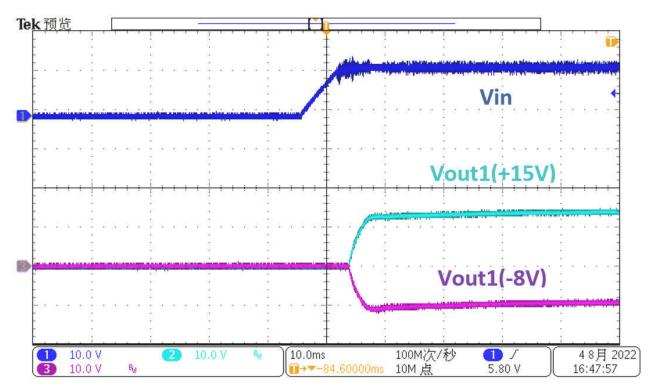
Figure 3-2. Channel A, +15 V, -8-V Output Start-Up Waveforms
