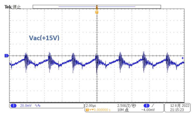
Figure 3-6. V<sub>OUT1</sub> +15-V Output Ripple, V<sub>IN</sub> = 12 V, I<sub>OUT1</sub> = 80 mA, I<sub>OUT2</sub> = 80 mA
