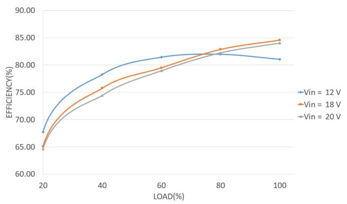
Figure 2-1. Average Efficiency for 10 V, 12 V, 18 V, 20 V
