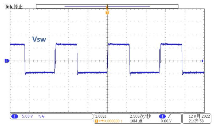
Figure 3-12. Switch Node Voltage,  $V_{IN}$  = 12 V,  $I_{OUT1}$  = 80 mA,  $I_{OUT2}$  = 80 mA
