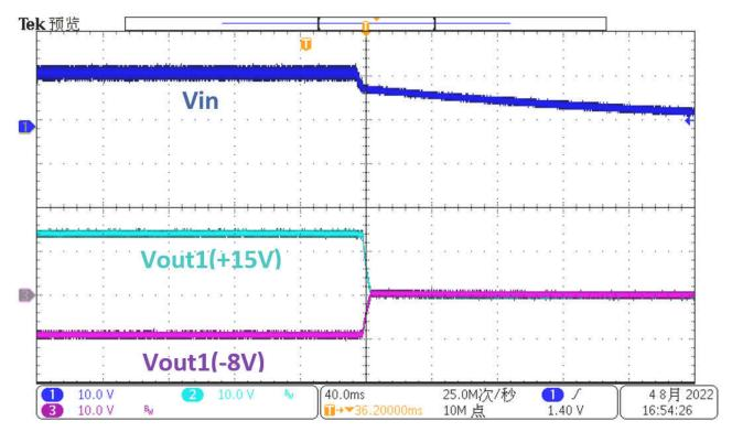
Figure 3-4. V<sub>OUT1</sub> Channel Power-Off Waveform of +15-V, 8-V Output With V<sub>IN</sub> = 12 V, I<sub>OUT1</sub> = 80 mA,  $I_{OUT2}$  = 80 mA
