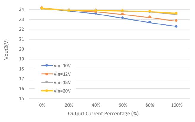
Figure 2-3. Isolated V<sub>OUT1</sub> and V<sub>OUT2</sub> Regulation With Same Percentage Current (Vout2)
