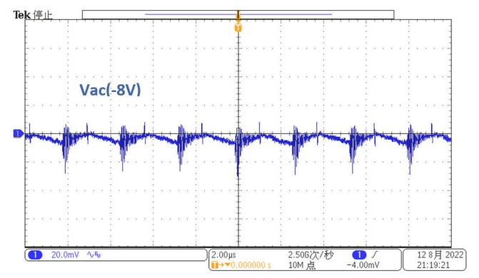
Figure 3-7.  $V_{OUT1}$  –8-V Output Ripple,  $V_{IN}$  = 12 V,  $I_{OUT1}$  = 80 mA,  $I_{OUT2}$  = 80 mA
