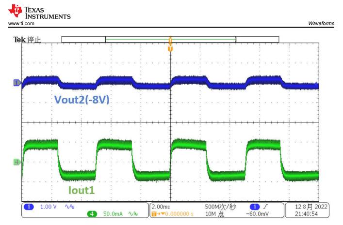
Figure 3-10. –8-V Output Load Transient at 12-V Input From 40 mA to 80 mA
