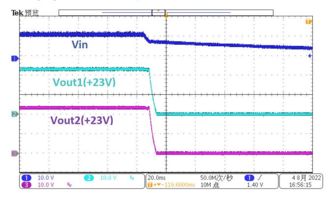
Figure 3-3. Two-Channel Power-Off Waveform of +23-V Output With V<sub>IN</sub> = 12 V,  $I_{OUT1}$  = 80 mA,  $I_{OUT2}$  = 80 mA
