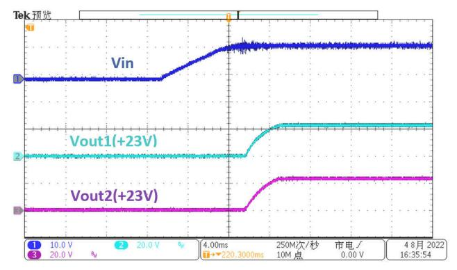
Figure 3-1. 12-V<sub>IN</sub> Dual-Channel Output Start-Up Waveforms
