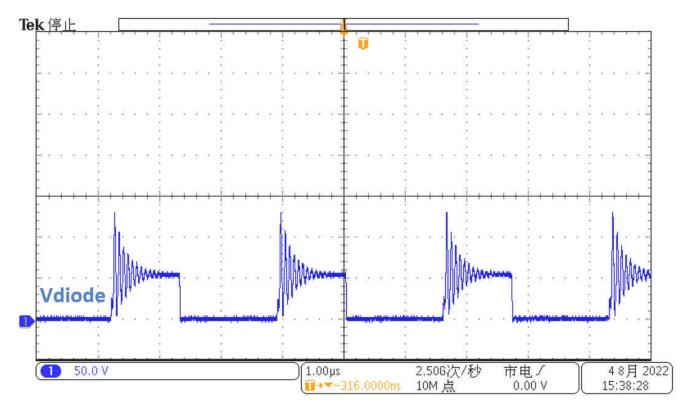
Figure 3-16. Channel A Diode Voltage Stress  $V_{IN}$  = 12 V,  $I_{OUT1}$  = 80 mA,  $I_{OUT2}$  = 80 mA
