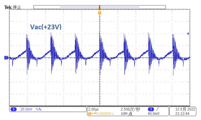
Figure 3-5.  $V_{OUT1}$  +23-V Output Ripple,  $V_{IN}$  = 12 V,  $I_{OUT1}$  = 80 mA,  $I_{OUT2}$  = 80 mA
