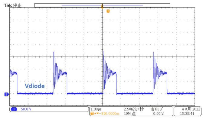
Figure 3-17. Channel A Diode Voltage Stress  $V_{IN}$  = 18 V,  $I_{OUT1}$  = 80 mA,  $I_{OUT2}$  = 80 mA
