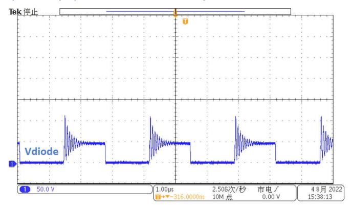
Figure 3-15. Channel A Diode Voltage Stress V<sub>IN</sub> = 10 V, I<sub>OUT1</sub> = 80 mA, I<sub>OUT2</sub> = 80 mA
