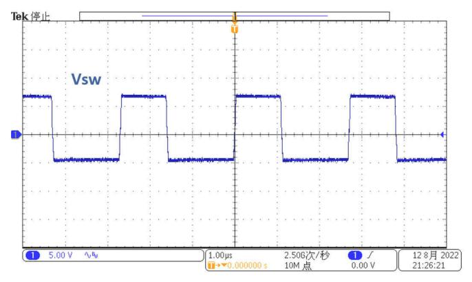
Figure 3-11. Switch Node Voltage,  $V_{IN}$  = 12 V,  $I_{OUT1}$  = 0 A,  $I_{OUT2}$  = 0 A
