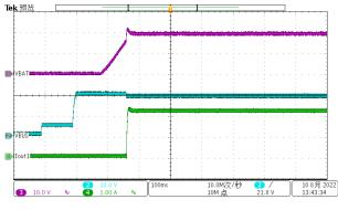
Figure 3-1.  $V_{\text{BUS}}$  20 V to  $V_{\text{BAT}}$  20-V Charge Mode
