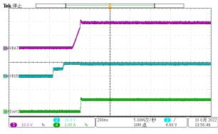
Figure 3-3.  $V_{\text{BUS}}$  9 V to  $V_{\text{BAT}}$  20-V Charge Mode
