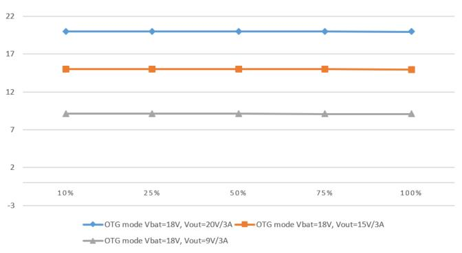
Figure 2-3.  $V_{\text{OUT}}$  Regulation of 5 V, 9 V, 15 V, and 20 V at OTG Mode
