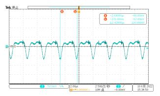
Figure 3-11. V<sub>BAT</sub> 18 V to 15 V, 3 A Full-Load Ripple Figure 3-12. V<sub>BAT</sub> 18 V to 20 V, 3 A Full-Load Ripple at OTG Mode at OTG Mode
