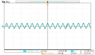
Figure 3-10. V<sub>BAT</sub> 18 V to 9 V, 3 A Full-Load Ripple at OTG Mode
