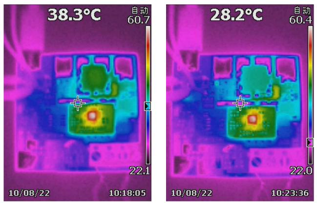
Figure 2-6. 9 V<sub>BUS</sub> and 20 V<sub>BAT</sub> Full Charging Mode Figure 2-7. 5 V<sub>BUS</sub> and 20 V<sub>BAT</sub> Full Charging Mode
