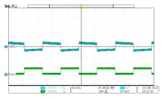
Figure 3-13.  $V_{\text{BAT}}$  18 V to 5  $V_{\text{BUS}}$  0.1 A to 3 A Load Dynamic
