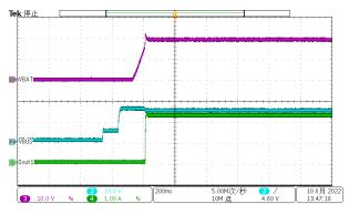
Figure 3-2.  $V_{\text{BUS}}$  15 V to  $V_{\text{BAT}}$  20-V Charge Mode
