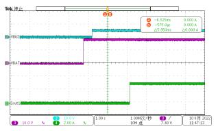
Figure 3-8. 18 V<sub>BAT</sub> to 5 V, 3 A Out OTG Mode
