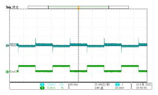
Figure 3-14. V<sub>BAT</sub> 18 V to 9 V<sub>BUS</sub> 0.1 A to 3 A Load Dynamic
