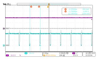
Figure 3-20. 20  $V_{BUS}$  to  $V_{BAT}$  21 V Charge Mode Working at Boost Mode
