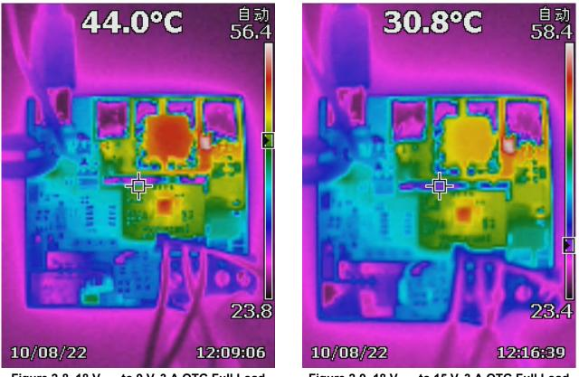
Figure 2-8. 18 V<sub>BAT</sub> to 9 V, 3 A OTG Full Load
