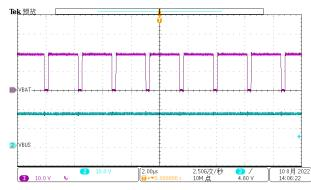
Figure 3-22. 20  $V_{\text{BUS}}$  to  $V_{\text{BAT}}$  19-V Charge Mode Working at Buck Mode
