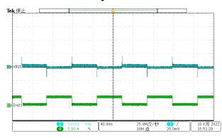
Figure 3-15. V<sub>BAT</sub> 18 V to 15 V<sub>BUS</sub> 0.1 A to 3 A Load Figure 3-16. V<sub>BAT</sub> 18 V to 20 V<sub>BUS</sub> 0.1 A to 3 A Load Dynamic
