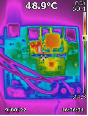
Figure 2-10. 18  $V_{\text{BAT}}$  to 20 V, 3 A OTG Full Load
