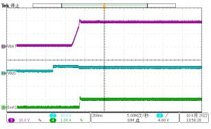
Figure 3-4.  $V_{\text{BUS}}$  5 V to  $V_{\text{BAT}}$  20-V Charge Mode
