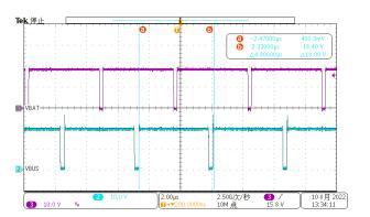
Figure 3-21. 20 V<sub>BUS</sub> to V<sub>BAT</sub> 20 V Charge Mode Working at Buck-Boost Mode
