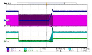
Figure 3-23. V<sub>BUS</sub> = 20 V, V<sub>BAT</sub> Short-Circuit Protection and Auto Recovery
