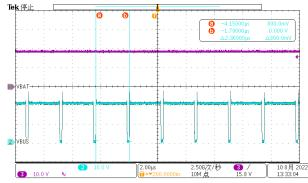
Figure 3-19. 21  $V_{\text{BAT}}$  to 20 V, 3 A Full Load OTG Mode Working at Buck Mode
