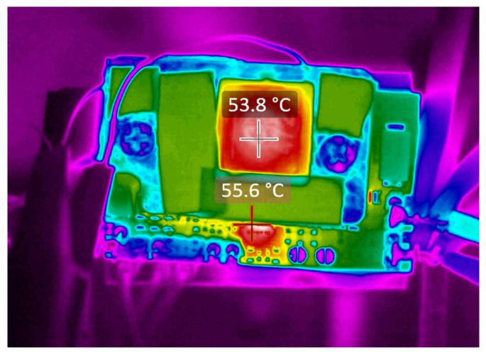
Figure 2-2. VBUS = 24 V, VBAT = 21 V, IBAT = 9.6 A, About 200 W, IC Temp = 55.6°C, Q1 FET = 53.6°C, IND Temp = 53.8°C (With Heat Sink, About 200 LFM Airflow)
