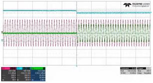
Figure 3-9. 230 VAC, 0% to 50% Load
