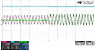
Figure 3-3. 120 VAC, 0% to 50% Load
