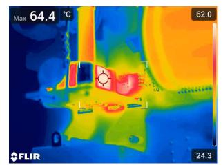
Figure 2-8. Common-Mode Choke and Hall Sensor
