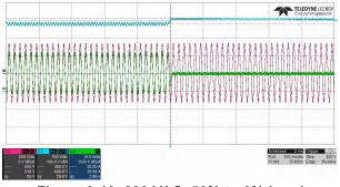
Figure 3-10. 230 VAC, 50% to 0% Load
