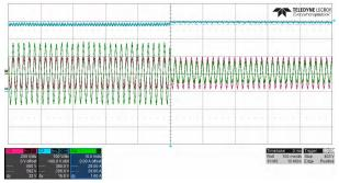
Figure 3-6. 120 VAC, 75% to 25% Load
