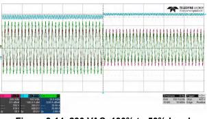
Figure 3-14. 230 VAC, 100% to 50% Load
