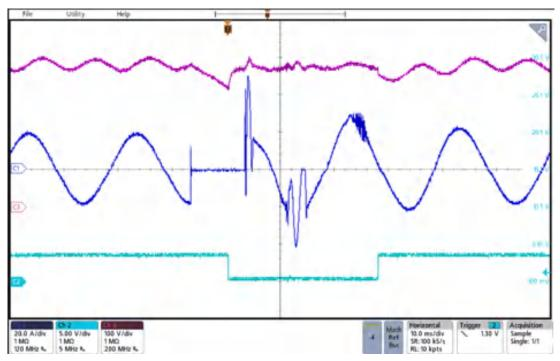
Figure 3-1. 230 VAC, 3 kW, 10-ms Drop, Return at 90 Degrees
