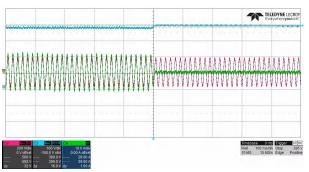
Figure 3-4. 120 VAC, 50% to 0% Load
