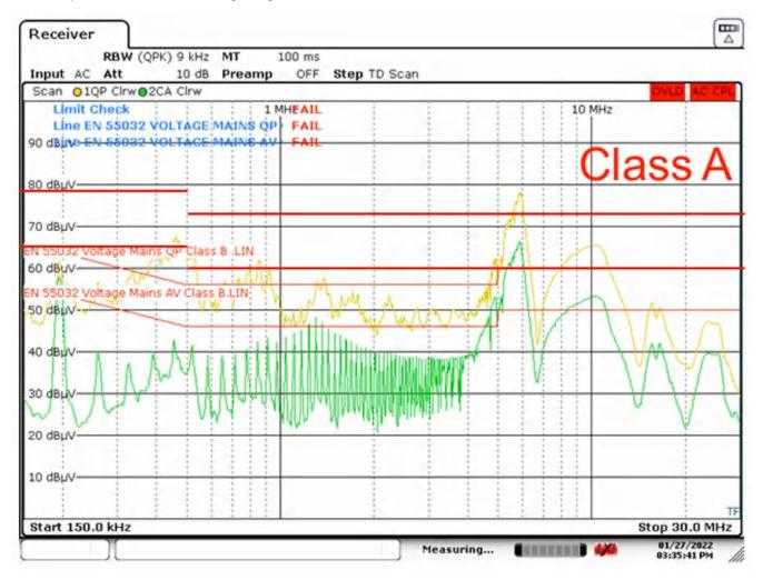
Figure 2-11. 230 VAC, Line, 400 W, X-cap: C44 = 1.97 µF, C45 = 3 µF
