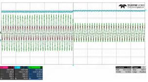
Figure 3-8. 120 VAC, 100% to 50% Load
