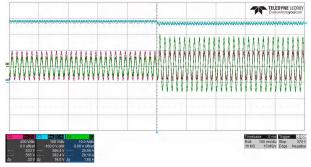
Figure 3-5. 120 VAC, 25% to 75% Load
