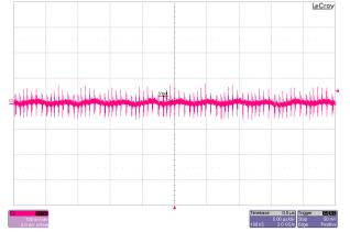
Figure 3-7. Output Voltage Ripple, No Load, PFM-Mode
