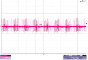
Figure 3-12. Output Voltage Ripple, 1-A Load, Zoomed Out, FPWM-Mode
