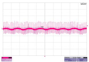
Figure 3-11. Output Voltage Ripple, 1-A Load, Zoomed Out, PFM-Mode
