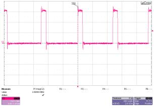
Figure 3-3. Switch Node Voltage, 1-A Load, PFM-Mode
