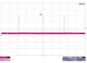
Figure 3-1. Switch Node Voltage, No Load, PFM-Mode
