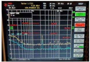
Figure 3-19. Conducted EMI Performance, 24-V Input, Low-Frequency Range
