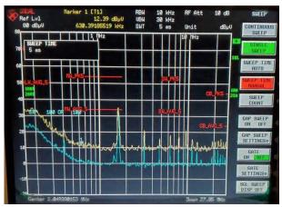
Figure 3-23. Conducted EMI Performance, 36-V Input, Low-Frequency Range
