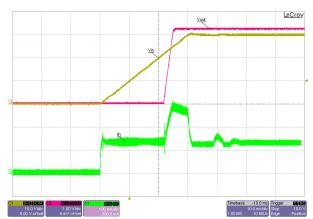
Figure 3-18. Start-up Into 1-A Constant-Current Load, 30-V Input, FPWM-Mode
