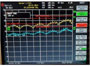
Figure 3-20. Conducted EMI Performance, 24-V Input, High-Frequency Range
