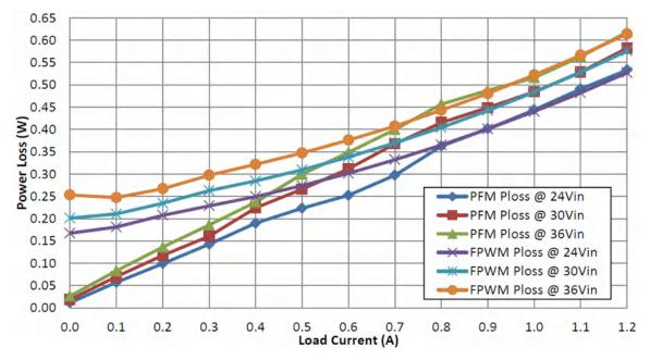
Figure 2-2. PMP22670 Converter Power Loss
