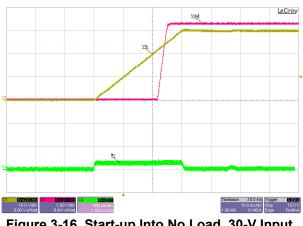
Figure 3-16. Start-up Into No Load, 30-V Input, FPWM-Mode
