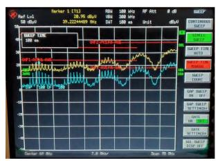
Figure 3-24. Conducted EMI Performance, 36-V Input, High-Frequency Range
