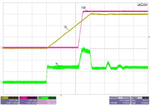
Figure 3-17. Start-up Into 1-A Constant-Current Load, 30-V Input, PFM-Mode
