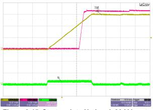
Figure 3-15. Start-up Into No Load, 30-V Input, PFM-Mode
