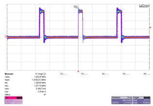
Figure 3-6. Switch Node Voltage, 1-A Load, Displaying Dither, FPWM-Mode
