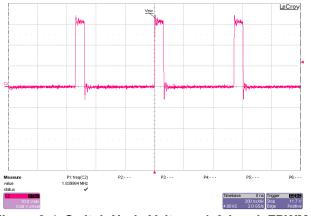
Figure 3-4. Switch Node Voltage, 1-A Load, FPWM-Mode
