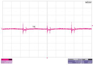
Figure 3-10. Output Voltage Ripple, 1-A Load, FPWM-Mode
