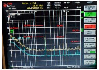
Figure 3-21. Conducted EMI Performance, 30-V Input, Low-Frequency Range
