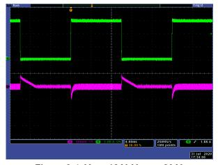
Figure 3-4.  $V_{IN}$  = 12 V,  $V_{OUT}$  = 20 V, I<sub>OUT</sub> from 0 A to 3 A
