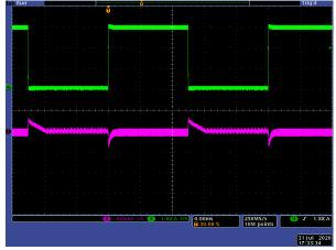
Figure 3-3.  $V_{IN}$  = 12 V,  $V_{OUT}$  = 15 V, I<sub>OUT</sub> from 0 A to 3 A
