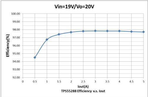
Figure 2-1. Efficiency of TPS55288
