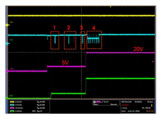
Figure 3-6. Start-up and PD Negotiation
