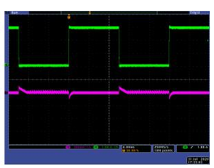
Figure 3-2.  $V_{IN}$  = 12 V,  $V_{OUT}$  = 9 V, I<sub>OUT</sub> from 0 A to 3 A
