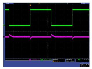
Figure 3-1.  $V_{IN}$  = 12 V,  $V_{OUT}$  = 5 V, I<sub>OUT</sub> from 0 A to 3 A
