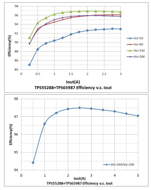
Figure 2-2. Efficiency of TPS55288 and TPS65987
