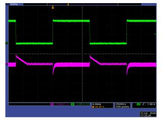
Figure 3-5.  $V_{IN}$  = 19 V,  $V_{OUT}$  = 20 V, I<sub>OUT</sub> from 0 A to 5 A
