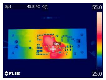
Figure 2-2. Bottom-Side Thermal Image, 120-V<sub>DC</sub> Input, 12 V at 400-mA Output
