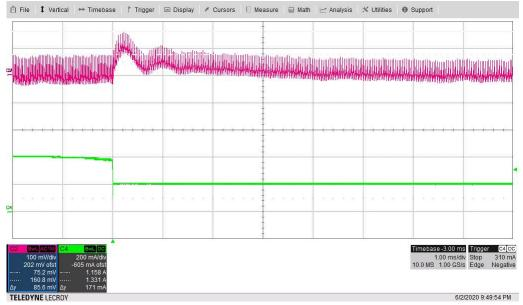
Figure 3-20. Load Transient, 12-V Output Voltage (AC Coupled) (V<sub>OUT</sub>: 100 mV/div, I<sub>OUT</sub>: 200 mA/div, 1 ms/div)
