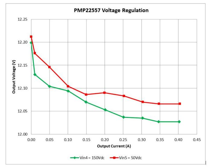
The following graph displays the measured output voltage at input voltages of 50  $V_{DC}$  and 150  $V_{DC}$ .
