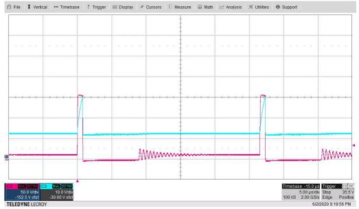
Figure 3-13. Switching Voltages (Vsnode: 50 V/div, D2-Cathode: 10 V/div, 5 µs/div)
