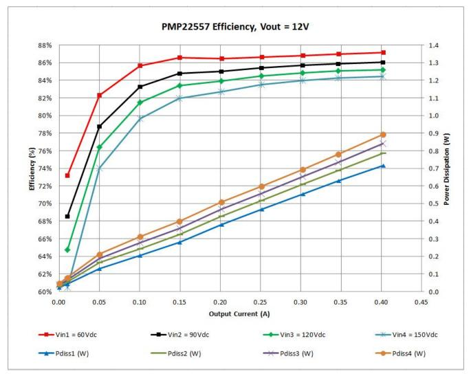
Figure 2-3. PMP22557 Efficiency, V<sub>OUT</sub> = 12 V
