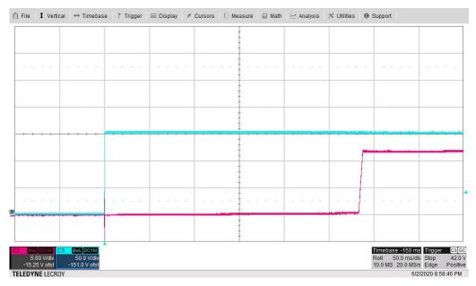
Figure 3-4. Output Voltage Start-up Waveform (VIN: 50 V/div, VOUT: 5 V/div, 50 ms/div)
