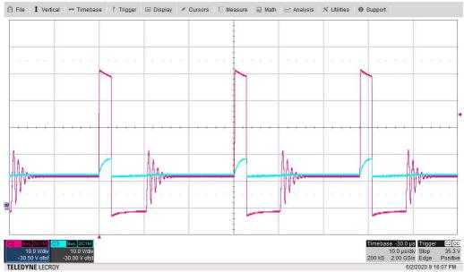
Figure 3-12. Switching Voltages (Vsnode: 10 V/div, D2-Cathode: 10 V/div, 10 µs/div)
