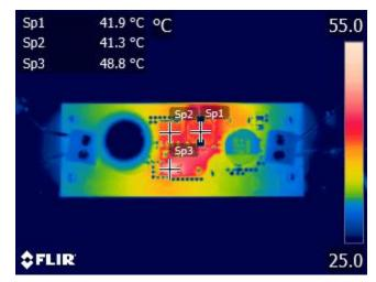
Figure 2-1. Top-Side Thermal Image, 120-V<sub>DC</sub> Input, 12 V at 400-mA Output
