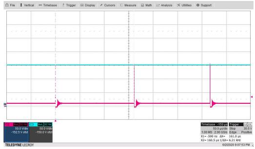
Figure 3-10. FET Switch Node Voltage (Vsnode: 50 V/div, V<sub>IN</sub>: 50 V/div, 50 µs/div)
