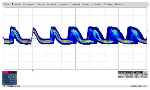
Figure 3-15. Output Voltage Ripple (AC Coupled) (V<sub>OUT</sub>: 50 mV/div, 20 µs/div)
