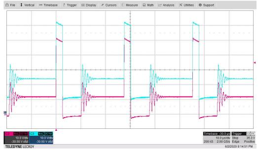
Figure 3-11. FET Switch Node Voltage (Vsnode: 10 V/div, D1-Cathode: 10 V/div, 10 µs/div)
