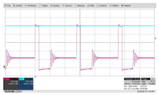
Figure 3-5. FET Switch Node Voltage (Vsnode: 10 V/div, V<sub>IN</sub>: 10 V/div, 10 µs/div)
