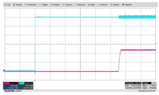
Figure 3-1. Output Voltage Start-up Waveform (V<sub>IN</sub>: 10 V/div, V<sub>OUT</sub>: 5 V/div, 50 ms/div)
