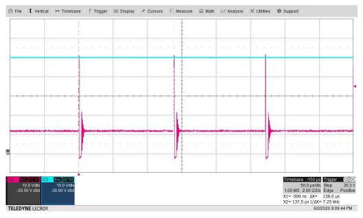
Figure 3-7. FET Switch Node Voltage (Vsnode: 10 V/div, V<sub>IN</sub>: 10 V/div, 50  $\mu$ s/div)
