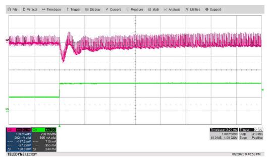
Figure 3-17. Load Transient, 12-V Output Voltage (AC Coupled) (V<sub>OUT</sub>: 100 mV/div, I<sub>OUT</sub>: 200 mA/div, 1 ms/div)
