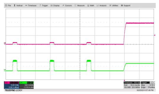
Figure 3-21. Short-Circuit Recovery (V<sub>OUT</sub>: 5 V/div, I<sub>OUT</sub>: 500 mA/div, 50 ms/div)
