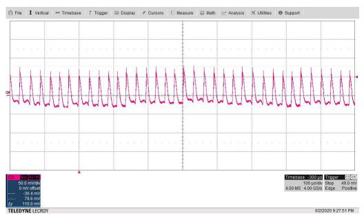
Figure 3-14. Output Voltage Ripple (AC Coupled) (V<sub>OUT</sub>: 50 mV/div, 100 µs/div)
