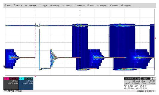
Figure 3-6. FET Switch Node Voltage (Vsnode: 10 V/div, V<sub>IN</sub>: 10 V/div, 10 µs/div)
