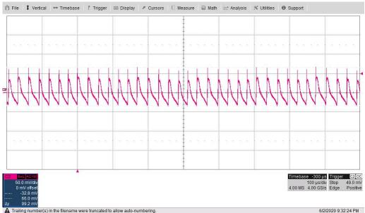
Figure 3-16. Output Voltage Ripple (AC Coupled) (V<sub>OUT</sub>: 50 mV/div, 100 µs/div)
