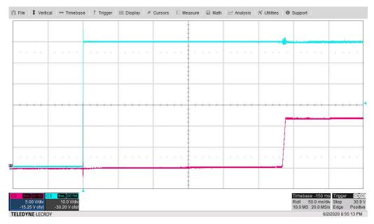
Figure 3-2. Output Voltage Start-up Waveform (VIN: 10 V/div, VOUT: 5 V/div, 50 ms/div)
