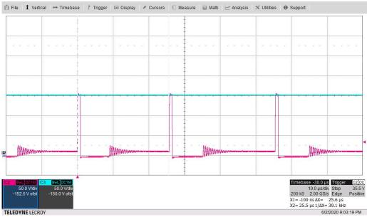
Figure 3-8. FET Switch Node Voltage (Vsnode: 50 V/div, V<sub>IN</sub>: 50 V/div, 10 µs/div)
