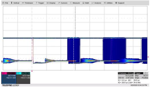
Figure 3-9. FET Switch Node Voltage (Vsnode: 50 V/div, V<sub>IN</sub>: 50 V/div, 10 µs/div)
