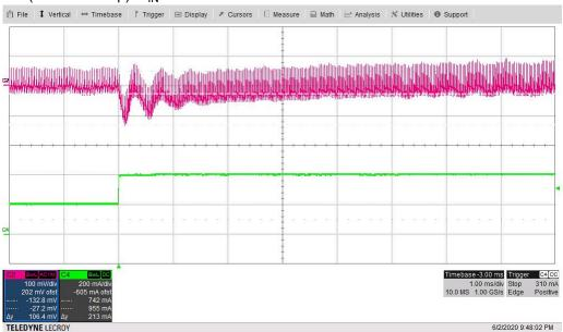
Figure 3-19. Load Transient, 12-V Output Voltage (AC Coupled) (V<sub>OUT</sub>: 100 mV/div, I<sub>OUT</sub>: 200 mA/div, 1 ms/div)
