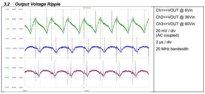
Figure 15 VOUT @ 6 V Input Voltage
