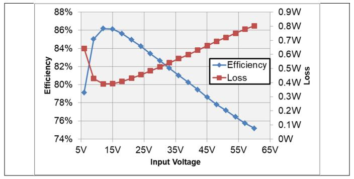
Figure 4 Efficiency and Loss vs Input Voltage
