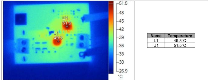
Figure 7 Thermal Image at 36 V Input Voltage
