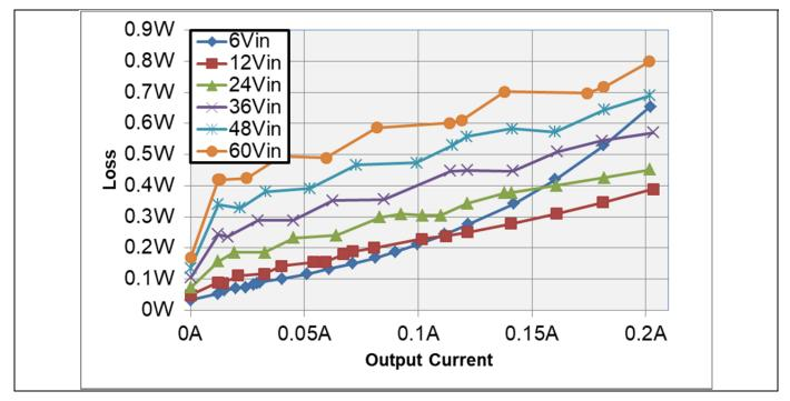
Figure 2 Loss vs Output Current
