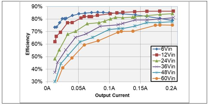
Figure 1 Efficiency vs Output Current
