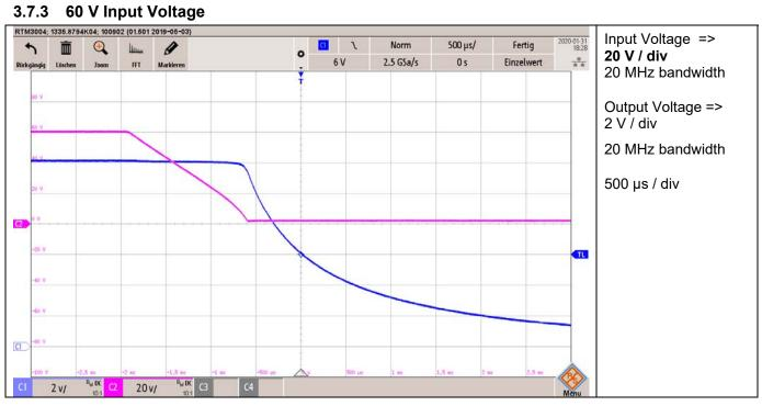
Figure 28 Shut-down @ 60 V Input Voltage
