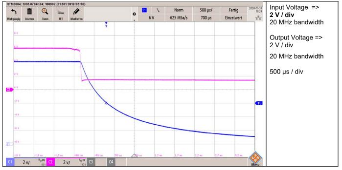
Figure 26 Shut-down @ 6 V Input Voltage
