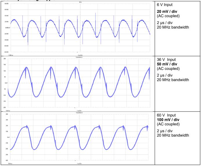
Figure 16 Input Voltage Ripple for 6 V, 36 V and 60 V Input Voltage
