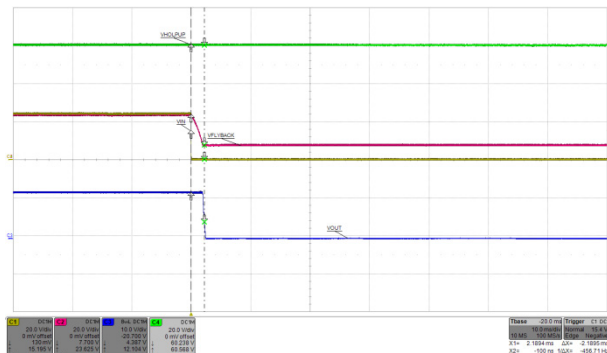
24Vin, 12Vout/1A, hot-unplug, hold-up disabled, 2ms holdup time.
