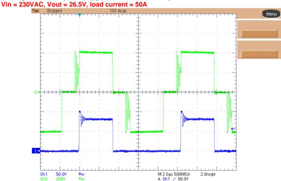
Ch3: Transformer voltage (pin 1-6) (200 V/div, 2 usec/div, 200 MHz BWL) Ch1: Sync. rectifier (Q21-Vds) (50 V/div, 200 MHz BWL)
