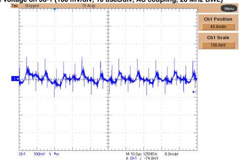
Ch1: Ripple voltage on J8-1 (100 mV/div, 10 usec/div, AC coupling, 20 MHz BWL)
