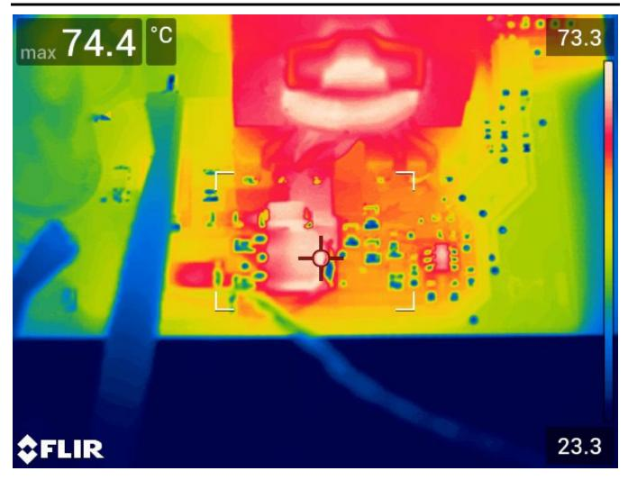
Figure 19. Q4 for UCC28742 flyback after 10 minute thermal soak at 150 Vdc input, loaded with 5 A on 12 Vdc rail
