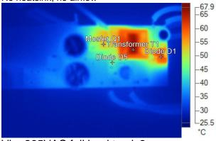
NameTemperatureTransformer T167.0°CDiode D544.5°CMosfet Q153.9°CDiode D160.3°C
