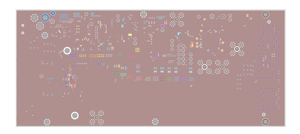
TEXAS INSTRUMENTS, INC. DAC38RF8x\_EVM PCB REV E LAYER 2 - GND
