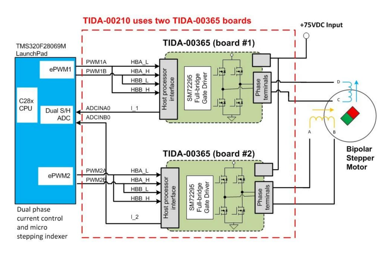
Note: The TIDA-00210 design is using two TIDA-00365 boards
