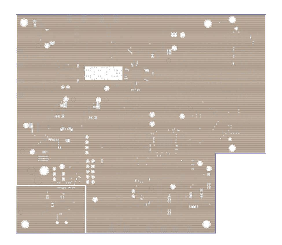
TEXAS INSTRUMENTS TSW14X500EVM PCB REV A L2 - GROUND PLANE
