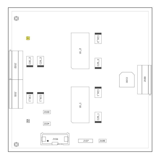
COMPONENTS MARKED 'DNP' SHOULD NOT BE POPULATED. ASSEMBLY VARIANT: 4-PHASE 90A
