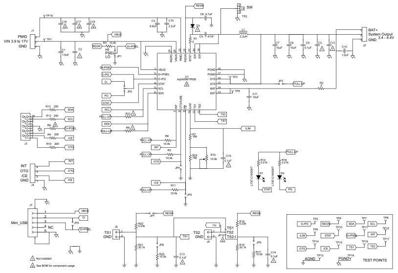
Figure 12. bq24x9xEVM Schematic
