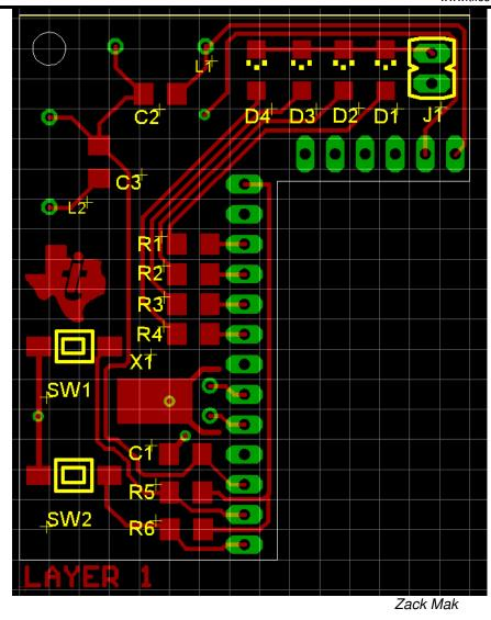
TI Designs: MSP430FW42x based Flow meter with Scan I/F
