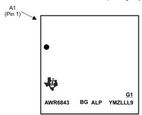
Figure 3-1. Example of Device Part Markings
