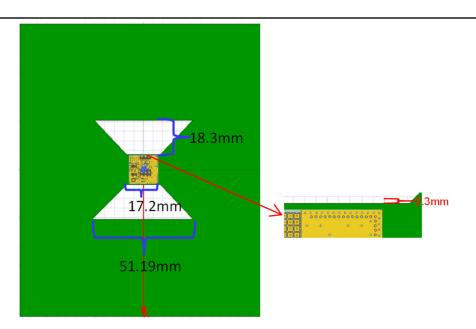
Figure 6-2. Large form factor board with trapezoidal cutout and PCB edge less than 0.3mm
