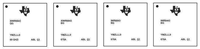
Figure 3-1. Example of Device Part Markings
